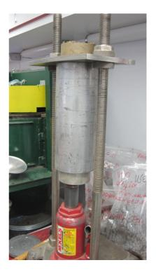
Figure 13. Extruding a statically compacted specimen
