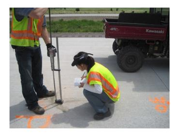
Figure 4. A dynamic cone penetrometer (DCP) in use
