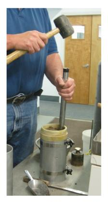
Figure 24. GeoTesting Express compaction process using a wooden dowel, rubber mallet, and split mold (photo courtesy of Nancy Hubbard)
