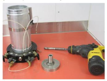
Figure 14. Split mold, steel platen (4 in. diameter), and vibratory hammer for compaction of granular materials
