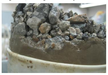
Figure 104. Interface of Iowa RPCC-Loess specimen after back saturated M<sub>r</sub> testing
