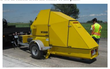
Figure 27. Falling weight deflectometer (FWD) in use on a concrete pavement surface
