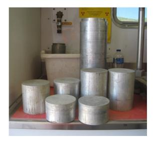
Figure 11. Aluminum spacers (4 in. diameter) used during static compaction
