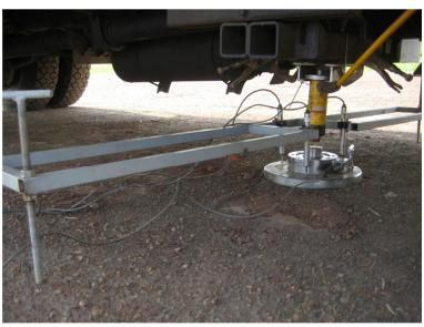
Figure 5. Plate load test (PLT) performed on subgrade
