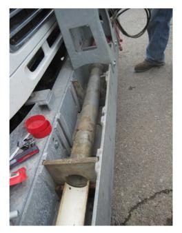
Figure 7. Shelby tube sampling; subgrade sample retrieval (left), sample extrusion (right)
