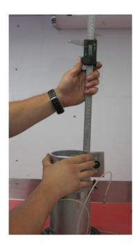
Figure 16. Verifying the thickness of each compacted layer with calipers
