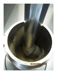
Figure 9. Soil compacted by kneading tamper foot
