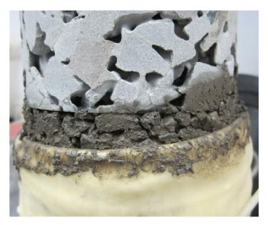
Figure 70. Pennsylvania US-22 composite material sample of CTB over class  ${\bf 2A~subbase~after~M_r~testing}$
