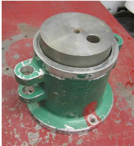
Figure 33. Application of surcharge pressure to sample in mold
