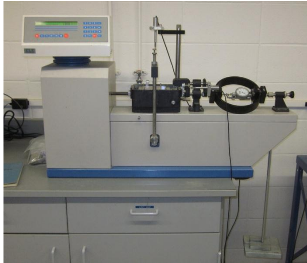
Figure 30. Drained direct shear test (ASTM D3080-04)
