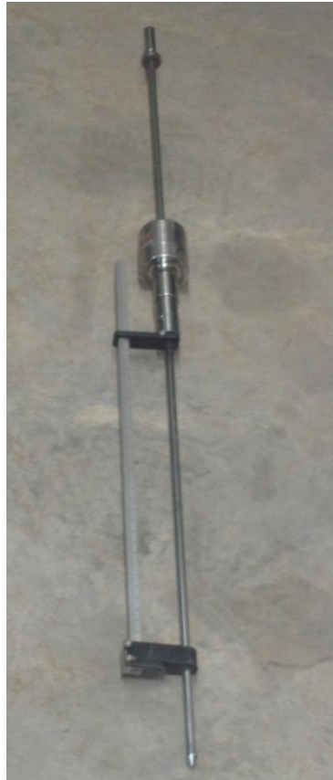
Figure 32. Dynamic cone penetrometer with 8 kg hammer (ASTM D6951-03)
