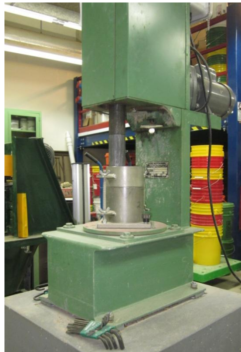
Figure 29. Standard Proctor test, method A (ASTM D698-00)
