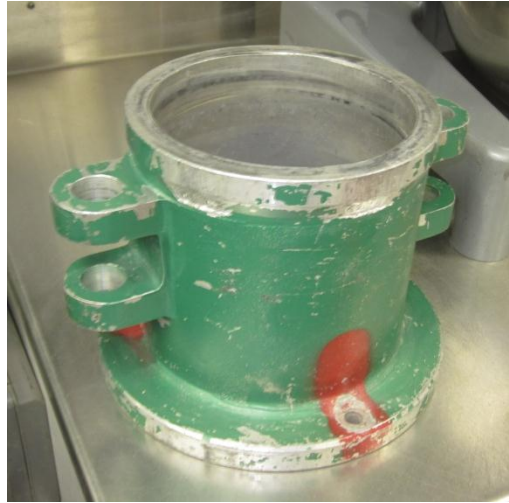
Figure 27. Relative density mold (ASTM D4253-83, D4254-83)
