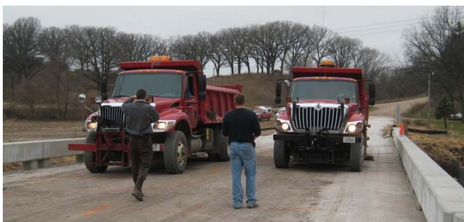
Figure 5-105. Live load test Run D (trucks in approximated driving lanes) for BC.
