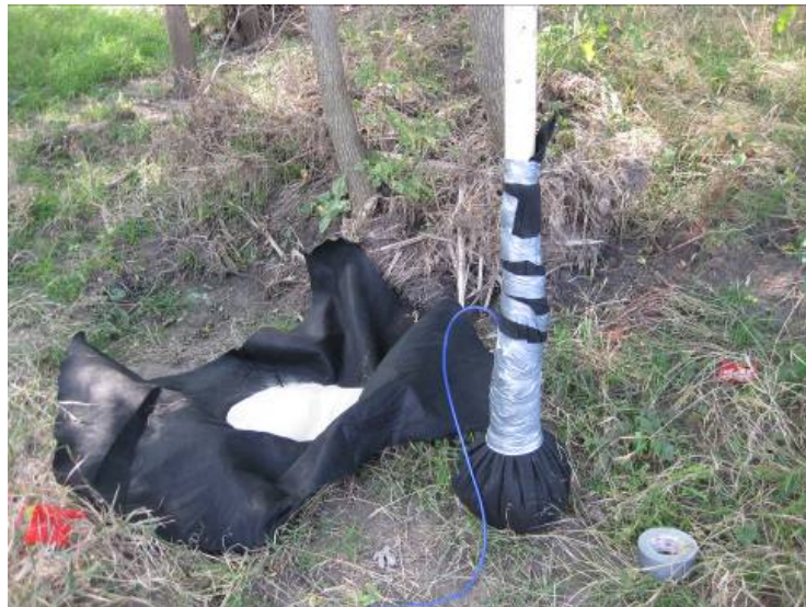
Figure 5-25. Piezometer assembly for water table monitoring.
