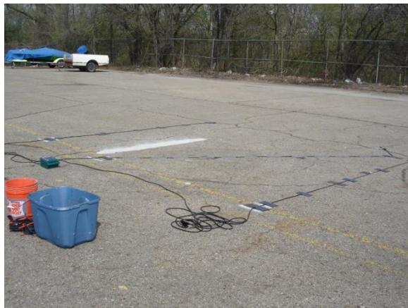
FIGURES F-4 and F-5 Z-configured road tube test setup with limestone aggregate ridge
