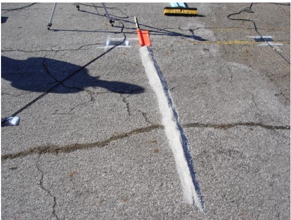
FIGURES F-4 and F-5 Z-configured road tube test setup with limestone aggregate ridge
