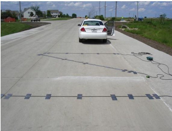
FIGURES F-7 and F-8 Z-configured road tube test bed with limestone aggregate ridge
