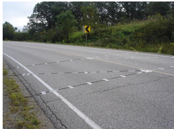
FIGURE G-5 Sta. C z-configured road tubes
