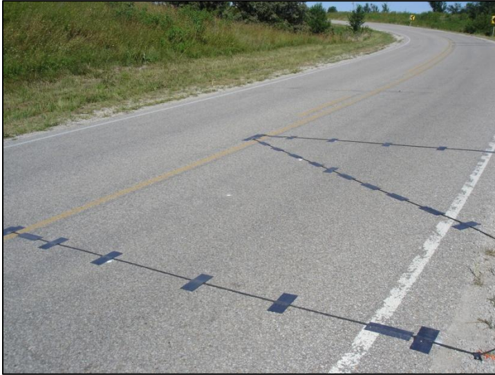
FIGURE 2-9 Pneumatic road tubes setup in a z-configuration
