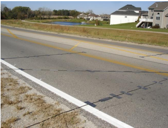
FIGURE G-17 Sta. D z-configured road tubes
