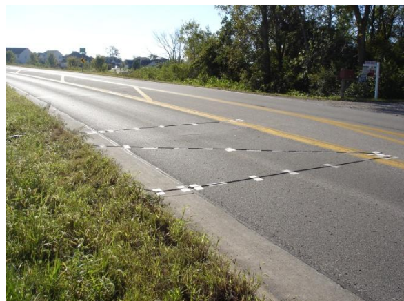
FIGURE G-15 Sta. B z-configured road tubes
