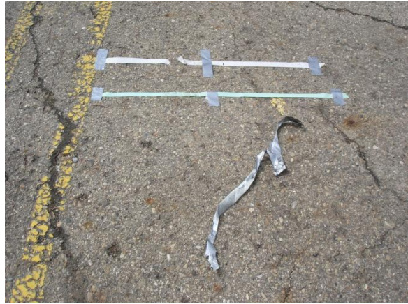
FIGURES F-1 and F-2 Tape test to determine tire lateral position (before and failure after)
