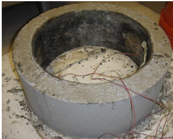
Figure 16 Configuration of restrained concrete ring samples.
