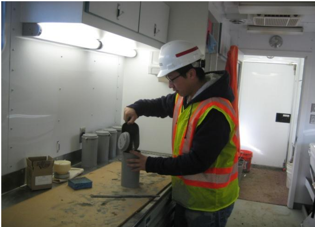
Figure 8 Preparing concrete cylinder samples.
