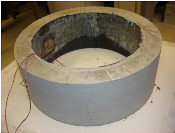
Figure 16 Configuration of restrained concrete ring samples.
