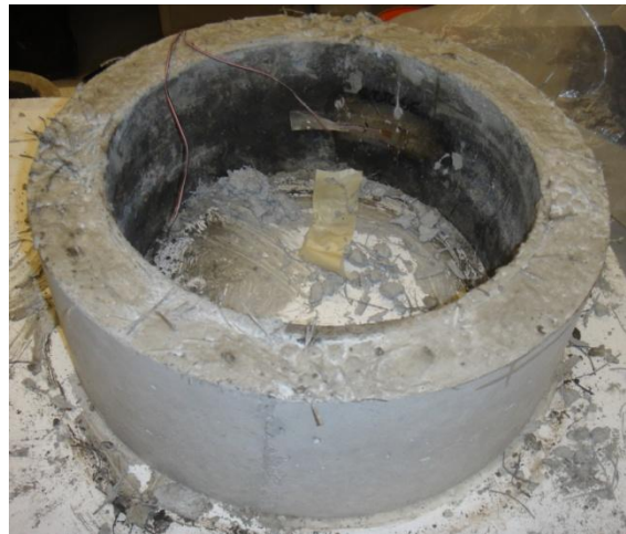
Figure 19 Configuration of restrained concrete ring samples.
