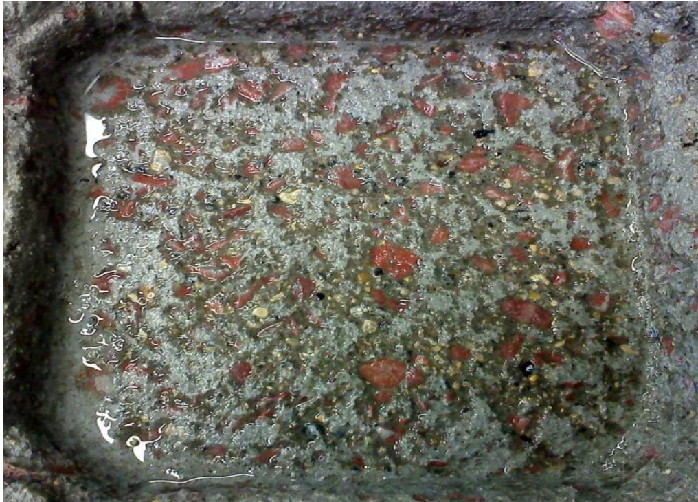
Figure 18 IA salt scaling sample after 50 th freeze-thaw cycle.
