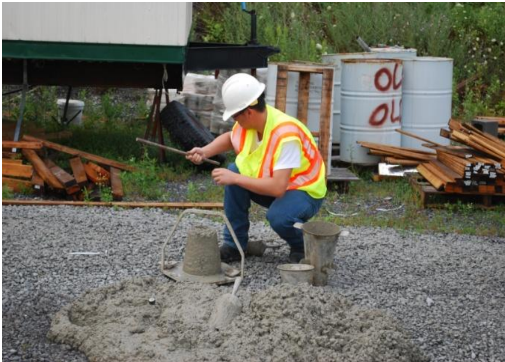
Figure 8 Concrete being tested by CP Tech Center technician PCC mobile lab.
