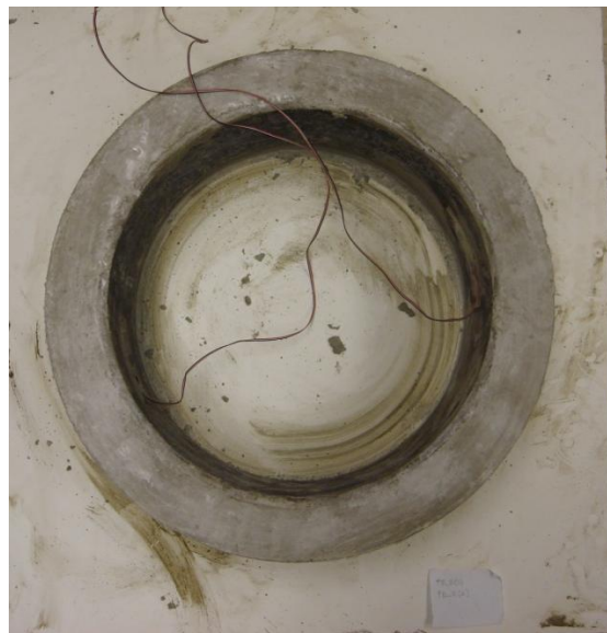
Figure 15 Configuration of restrained concrete ring samples.
