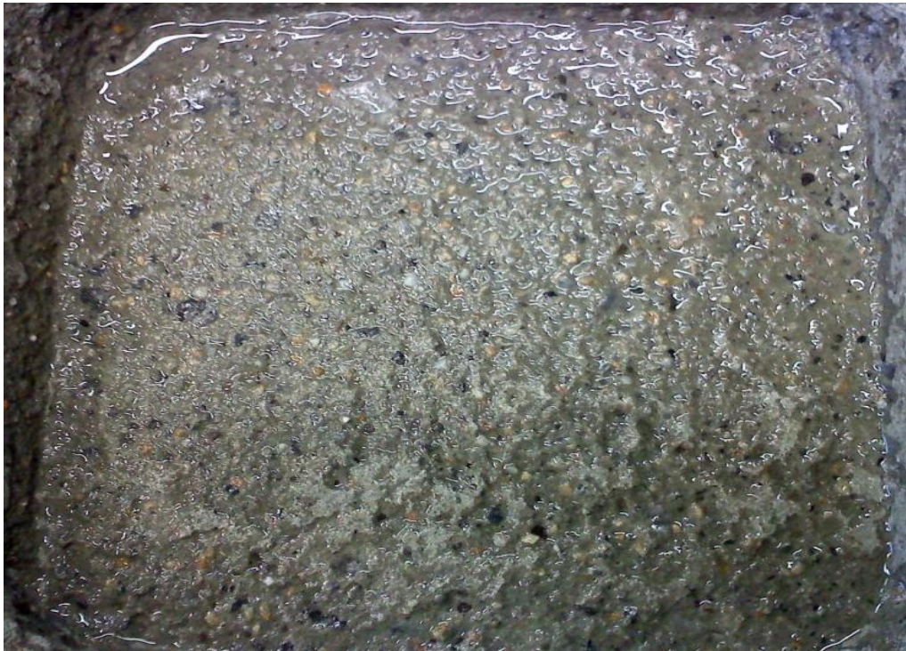
Figure 23 PA salt scaling sample after 50 th freeze-thaw cycle.
