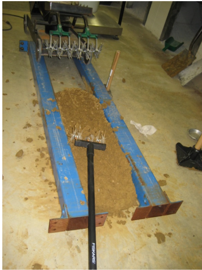
Figure 15. 4 inch depth clay soil bed with manual tiller.
