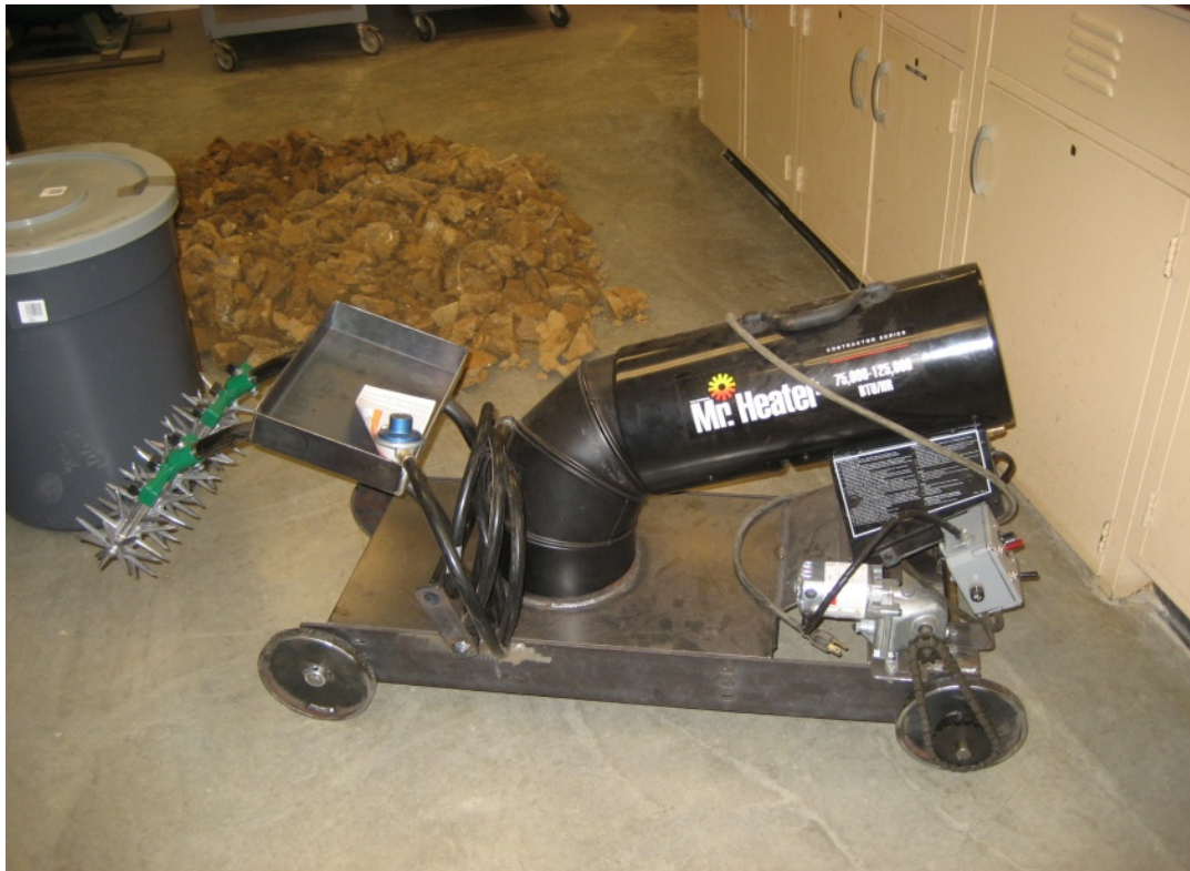
Figure 4: PRO-SD Laboratory Scale Propane Soil Drying Device
