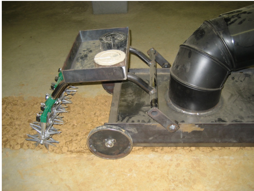
Figure 13. PRO-SD in operation over a 1.5 inch soil depth and mechanical tilling.
