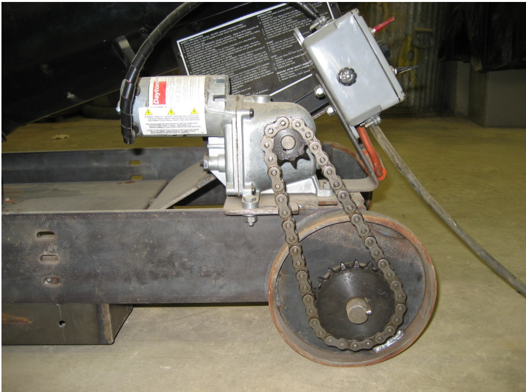
Figure 6. PRO-SD side view of the electric motor and drive chain.
