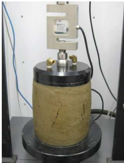
Figure 16. Unconfined compressive test on gyratory compacted specimen
