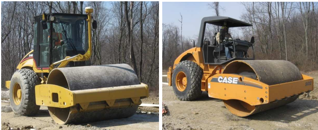
Figure 43. Caterpillar (left) and Case (right) smooth drum rollers used in the West Virginia site
