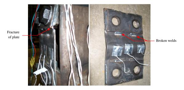
Figure 8 Redesigned structural fuse plate highlighting fracture of the plate and welds
