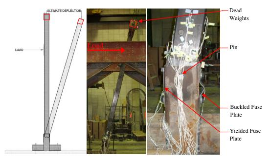
Figure 3 Schematic of test specimen and maximum deflection of laboratory test with buckled structural fuse plate
