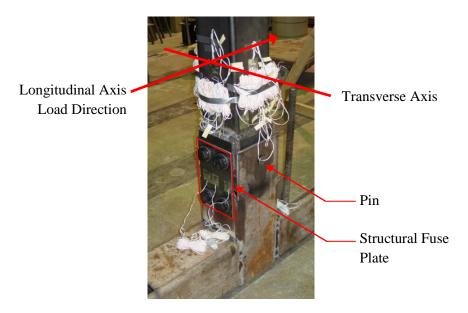
Figure 1 Connection of two main HSS segments using a pin and structural fuses
