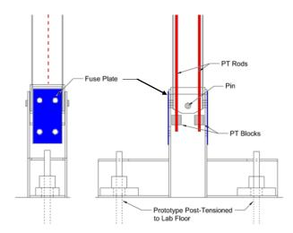
Figure 2 Schematic of prototype specimen highlighting post tensioning, fuses, and pin connection
