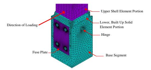
Figure 9 Finite element model
