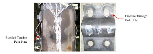
Figure 5 Post-test buckled structural fuse plates with fracture of tension fuse plate highlighted
