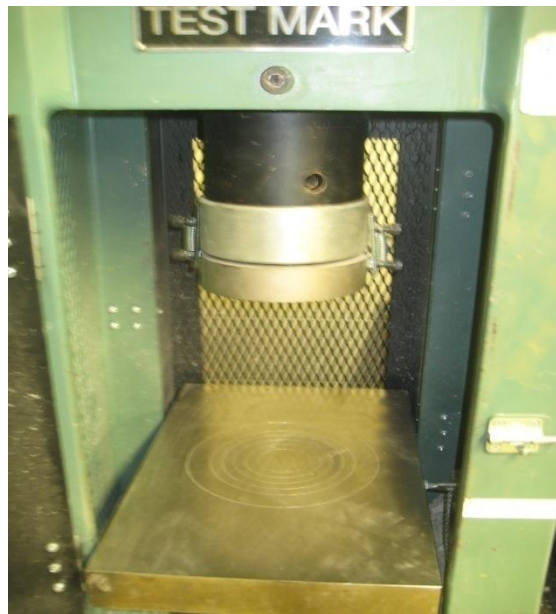
Figure 3 - 8. Test Mark compressive strength testing equipment
