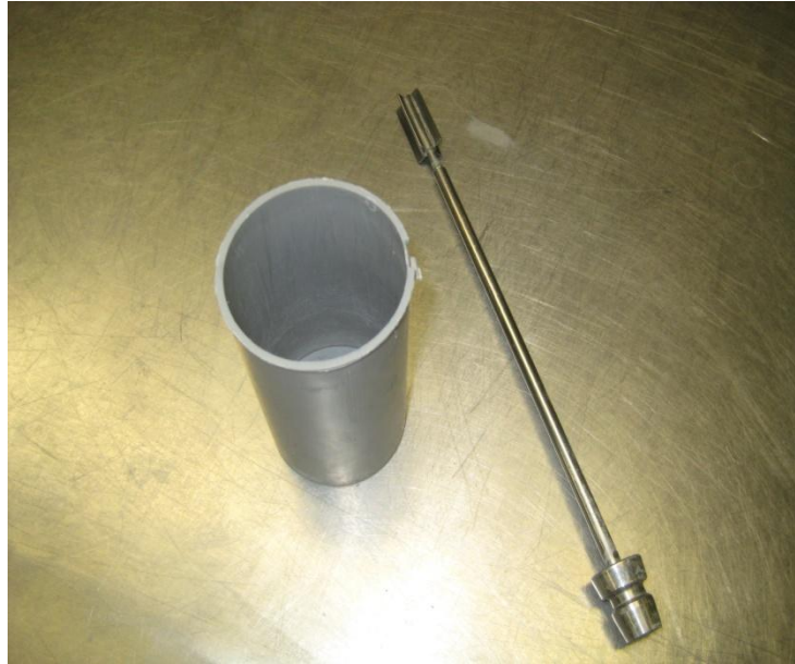
Figure 3 - 3.Vane and cylinder for rheometer
