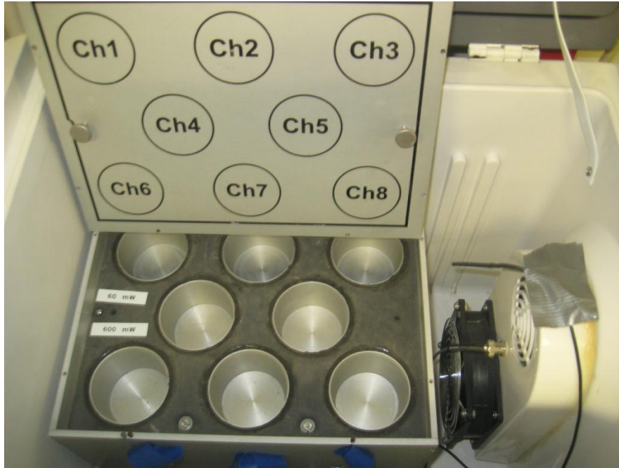
Figure 3 - 7. The unit of isothermal calorimeter
