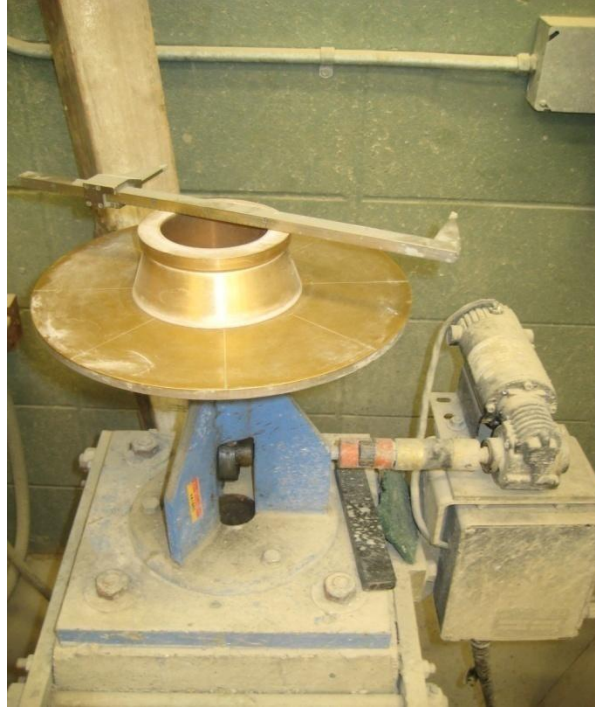
Figure 3 - 6. Flow table equipment
