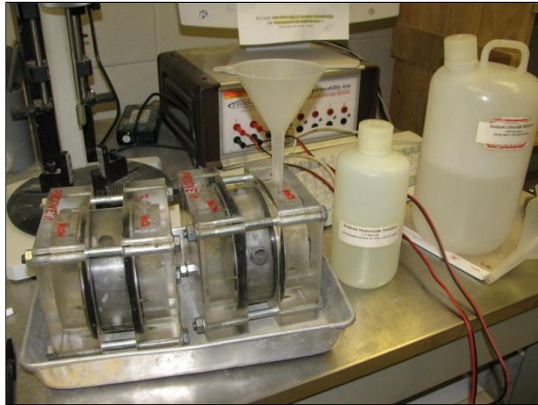
Figure 24. Rapid chloride penetration equipment
