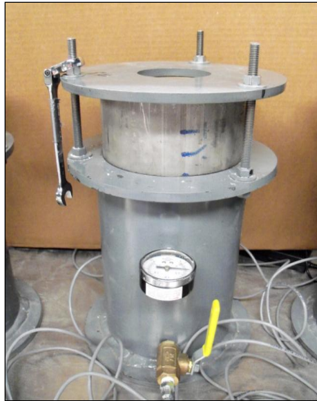
Figure 26. Air permeability equipment
