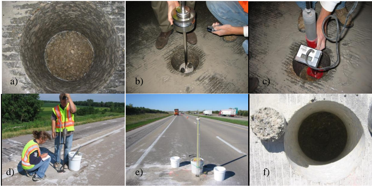
Figure 2.1. Field tests: a) 250 mm core hole; b) LWD; c) Clegg impact hammer; d) DCP; e) in situ Mn/DOT permeameter; f) a sample collected by coring by from a 250 mm core hole
