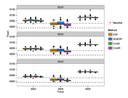
Figure 2.14 July Pool Elevation: The dot-dashed line minimum threshold of 1 MAF (6049.15 ft) and the dashed line is the minimum operating pool elevation for NIIP (5,990 ft).
