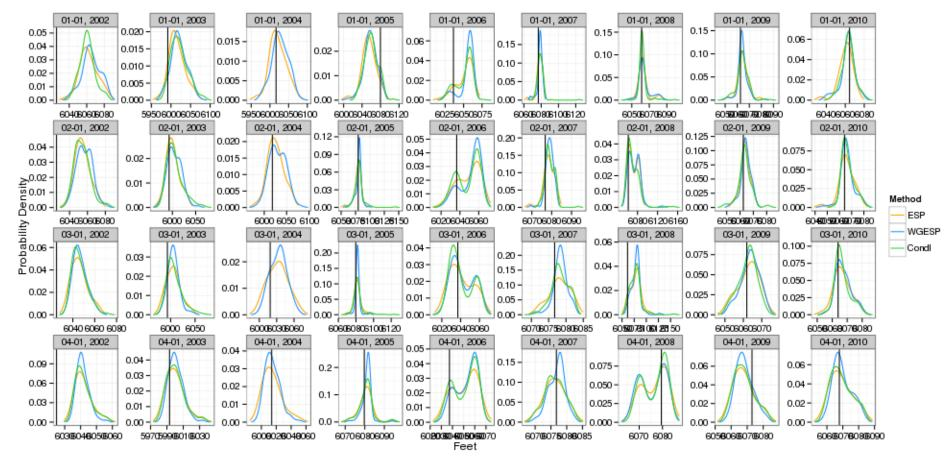
Figure 2.10 July Pool Elevation PDFs. The black vertical line is the baseline value calculated at each lead time for each year.
