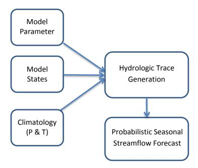
Figure 1.1 Ensemble Streamflow Prediction (ESP) Schematic
