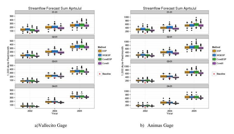
Figure 1.19 CHPS Streamflow Forecasts for ESP, WGESP, and CondI for 2002, 2004, and 2005. CondII means the SWG was conditioned using the winter precipitation and spring temperature forecasts. The remaining gages can be found in Appendix A.
