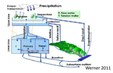
Figure 1.2 Sacramento Soil Moisture Accounting Model Schematic
