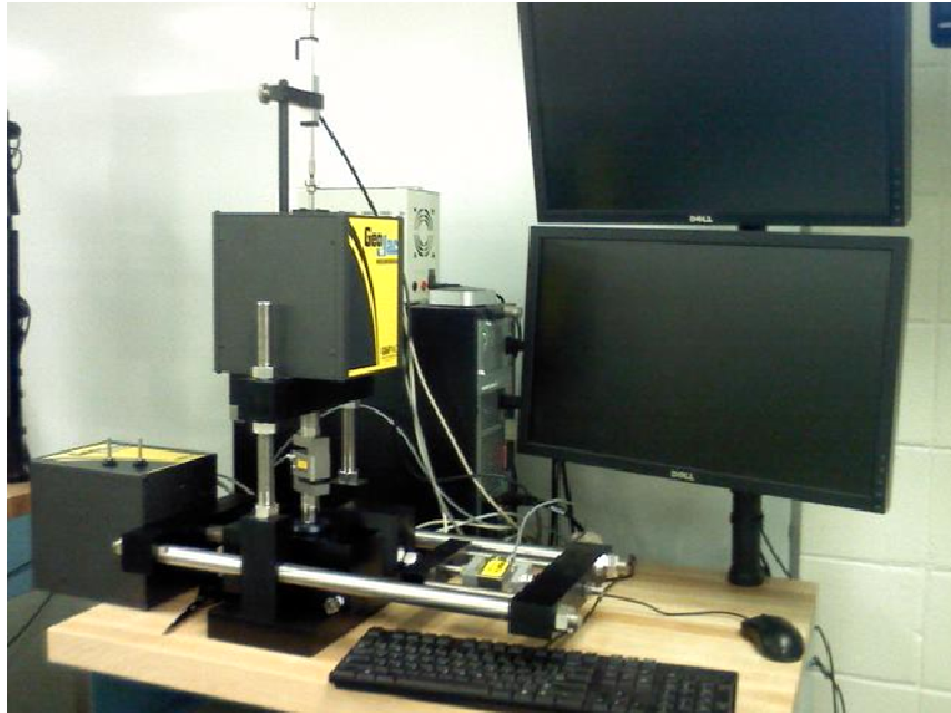
Figure 4.6: GeoTAC DigiShear direct shear apparatus
