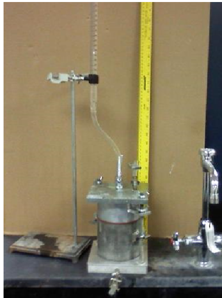
Figure 4.5: ELE International, Inc. model 25-0618 (K-610A) permeameter
