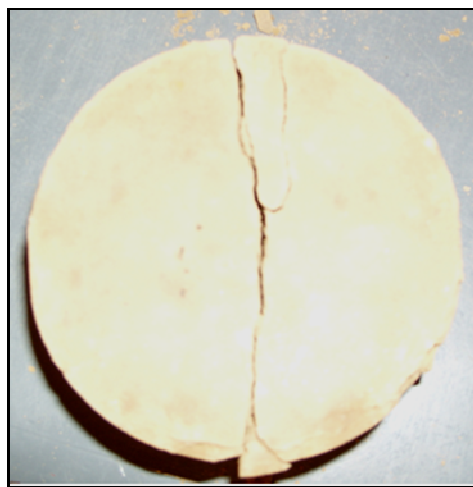
Figure 3.9: Failure mode of an indirect tensile test specimen with RAS
