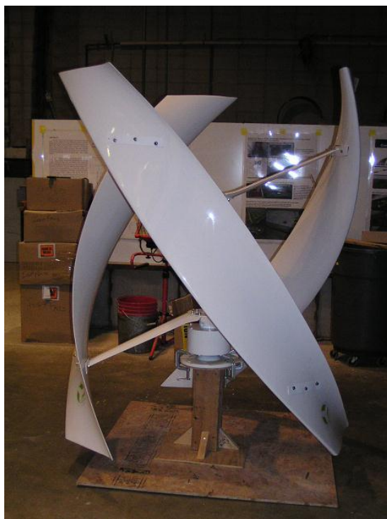
Figure 37: Full Assembly of 600 watt VAWT
