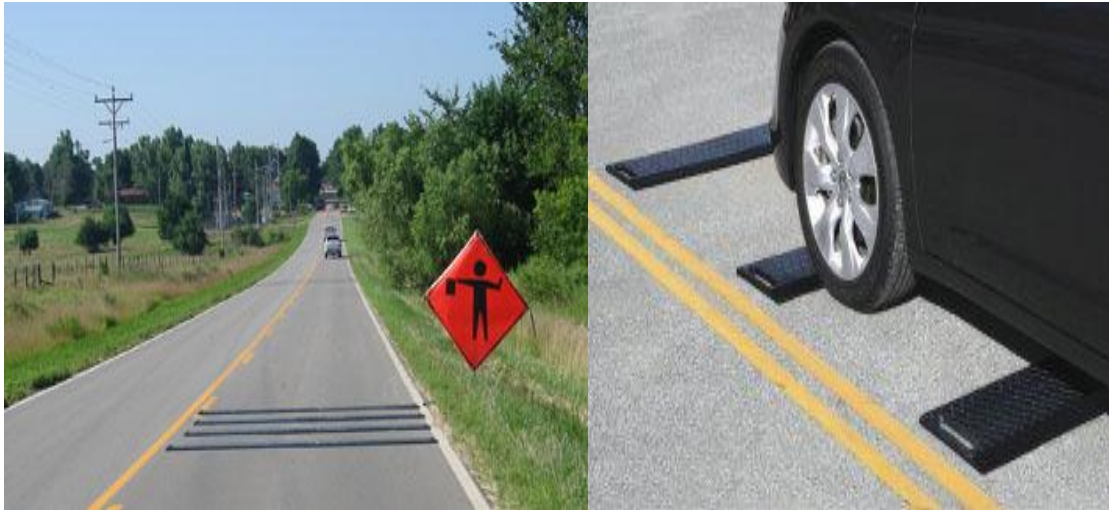
Figure 4. Portable temporary rumble strips being field tested near Perry, Kansas
