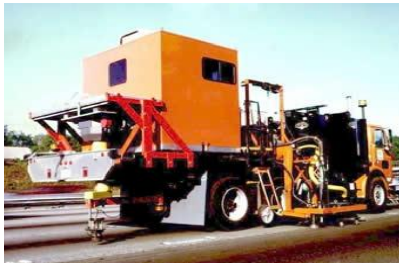
Figure 6. Automated Pavement Crack Sealer
