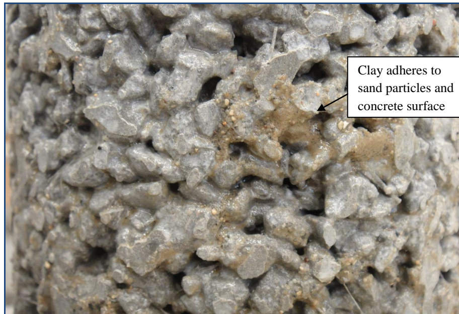
Figure 4-6. Specimen After Exposure to Clayey Silty Sand (Adapt from [28])
