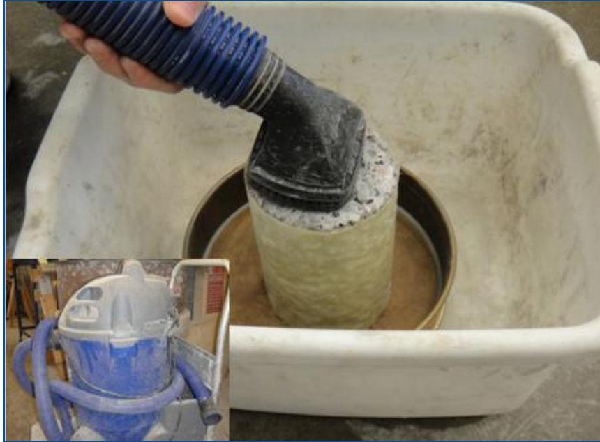
Figure 3-7. Vacuuming the Clogged Specimen
