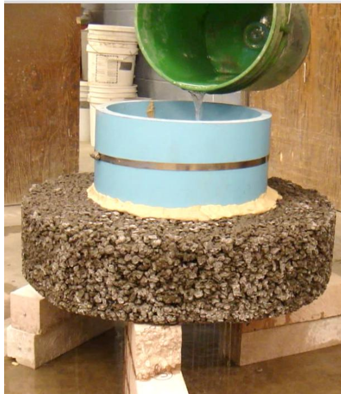
Figure 5-1. Laboratory Clogging Testing by Using ASTM C 1701 Standard “Standard Test Method for Infiltration Rate in Place Pervious Concrete”
