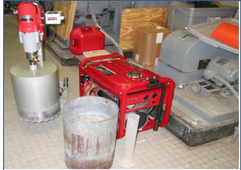
Figure 2-11. Embedded Single-Ring Infiltrometer Method (Adopted from [39])
