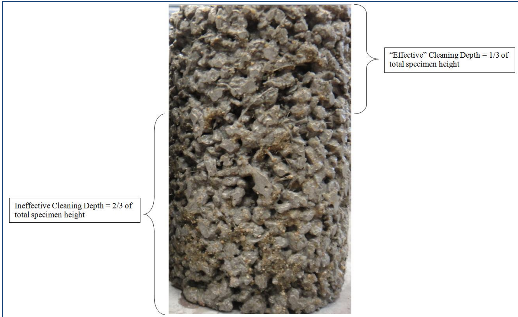
Figure 4-22. Cylinder Specimens Subjected to Clay Silty Sand Sedimentation and Cleaned by Pressue Washing and Vacuuming
