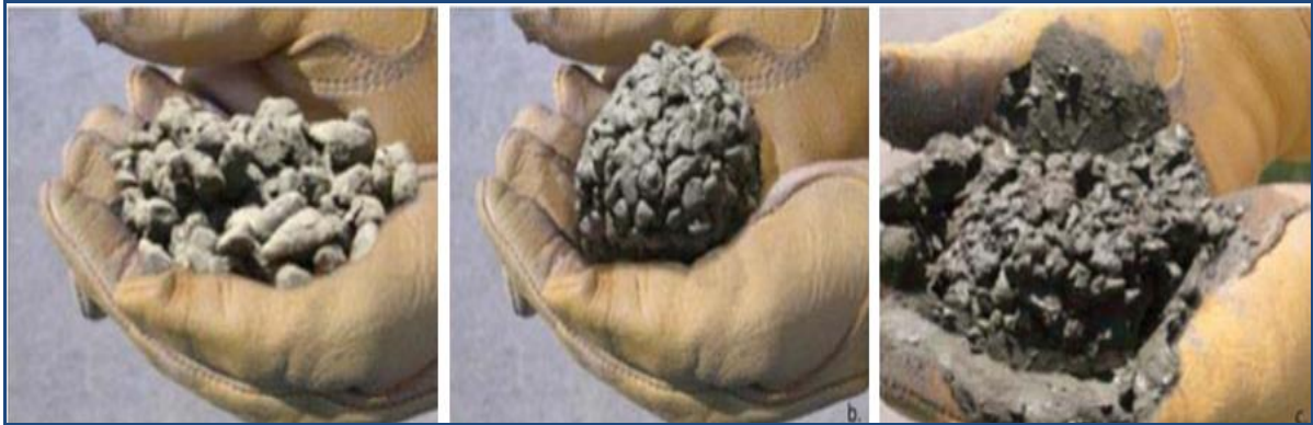
Figure 2-2. Samples of Pervious Concrete with Different Water Contents, Formed into A Ball (a) too little water, (b) proper amount of water, and (c) too much water (Adopted from [24])
