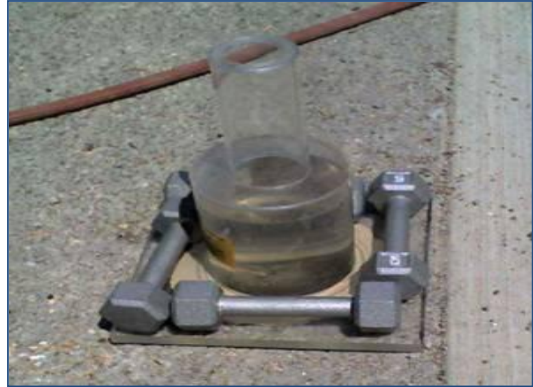
Figure 2-12. Field Permeameter Setup
