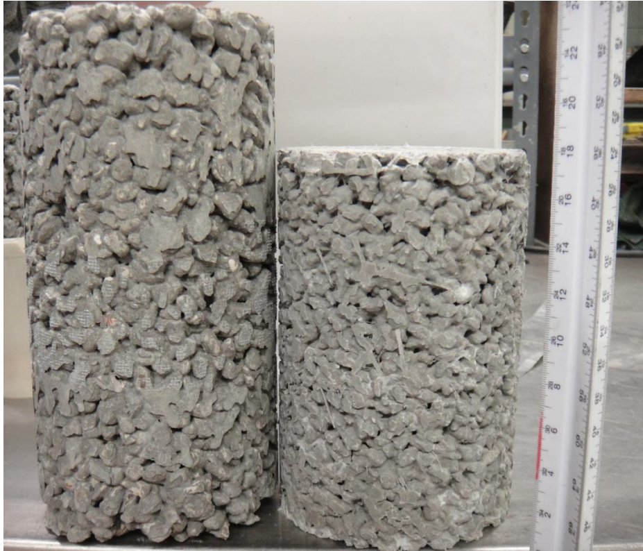
Figure 3-2. Untrimmed Specimen (Left) and Trimmed Specimen (Right)
