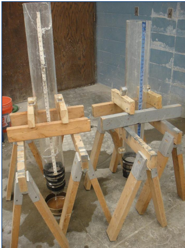
Figure 3-9. Falling Head Permeability Testing Used in This Study
