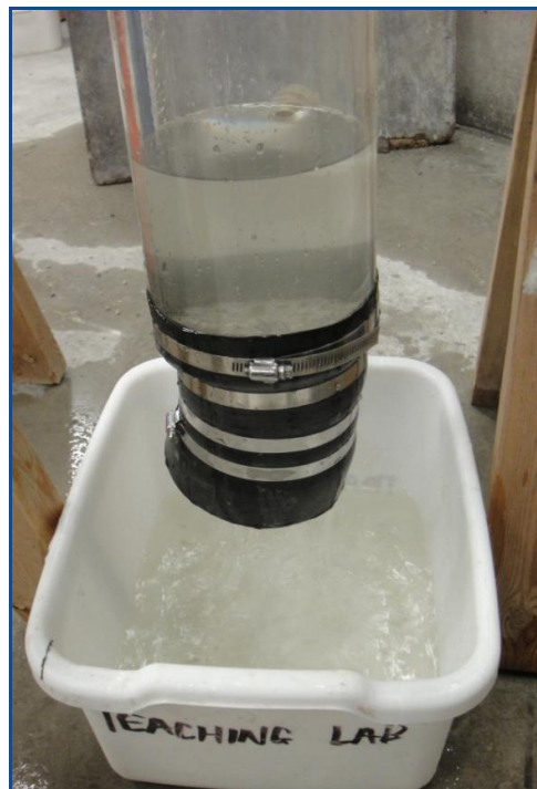
Figure 4-11. Sand Sedimentation Test is in Progress
