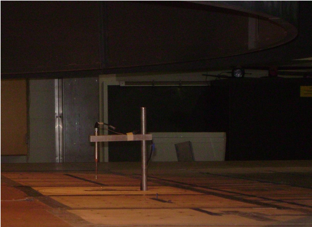
FIGURE 3-6 COBRA PROBE SET UP FOR WIND VELOCITY MEASUREMENTS
