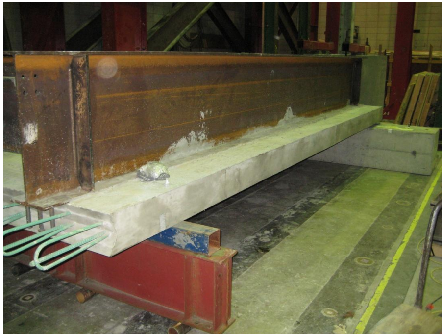
Figure 3.12. Completed Deck Module
