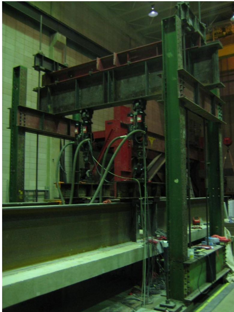
Figure 3.21. Load Frame for Service Level Testing
