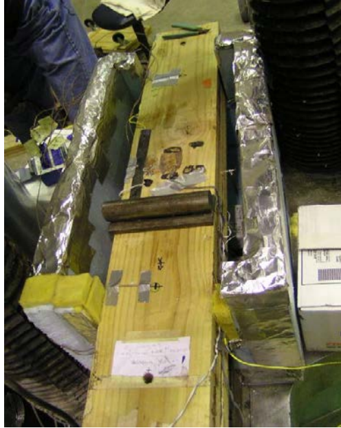
Figure 6.30. Cold and Sustained Loading Test: Placing the Specimen in the Cold Box
