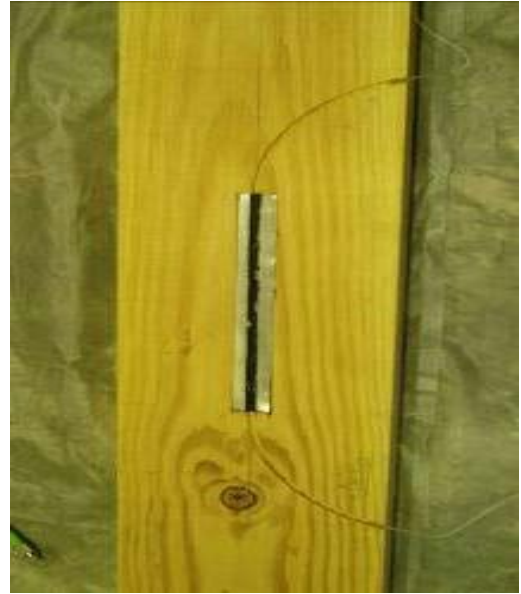
(b) Installed internal CS-SS Loctite 426 package
