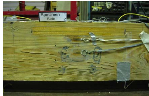
(b) After Hot and Sustained Loading
