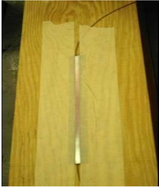
(a) Bonded backing material and tape to host the FBG sensor
