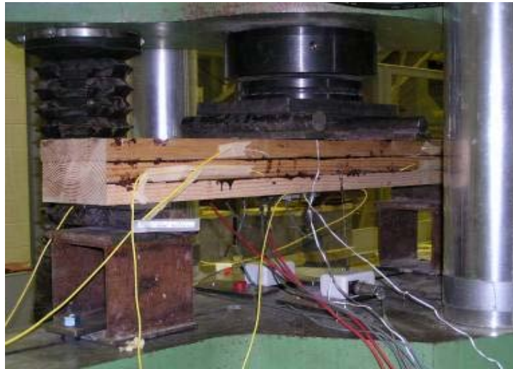
Figure 6.25. Small Scale Glulam Specimen with Structural Package and Test Setup
