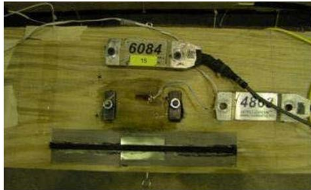
Figure 6.23. Specimens with Structural Packages: FBG Sensor, Foil Strain Gage and Strain Transducers
