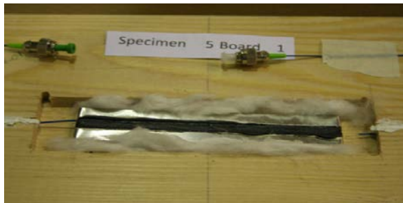
(a) Laminate 2: CS-SS structural package with cotton fiber
