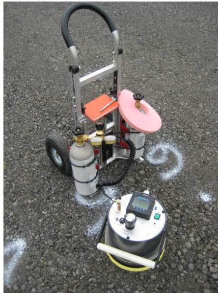
Figure 4. Gas permeability test used in the field
