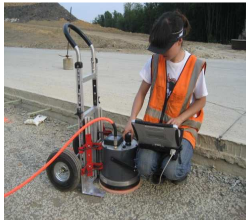
Figure 5. Gas permeability test used in the field with air compressor
