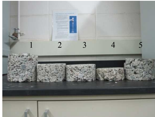
Figure 100. Compaction of specimens of CTB I-96 Michigan
