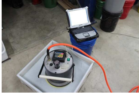
Figure 107. Gas permeability test of thin layers test
