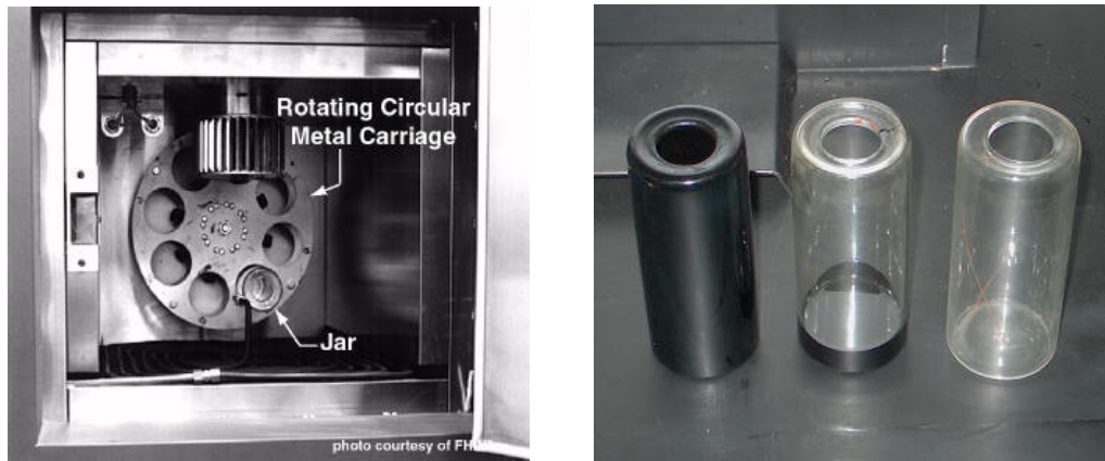
Figure 3.7 The RTFO Chamber and the Sample Cylinders
