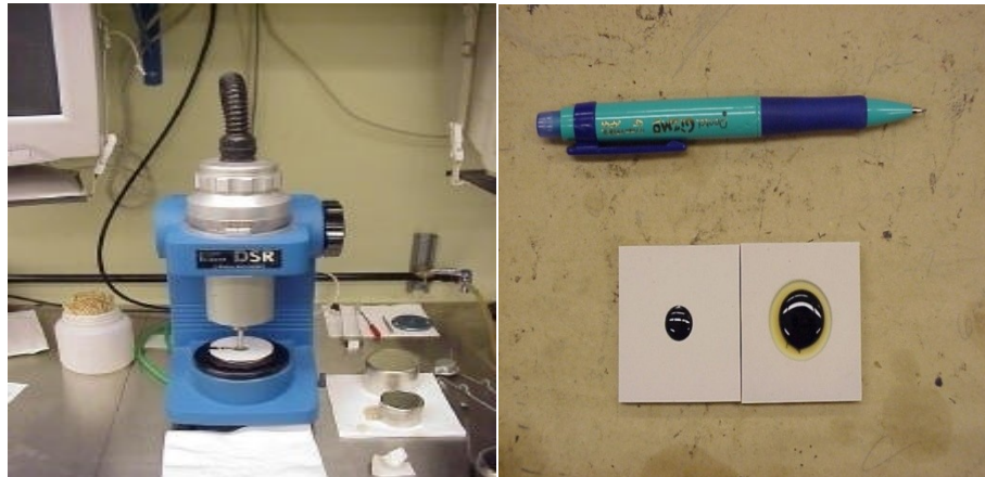
Figure 3.9 Dynamic Shear Rheometer machine and the sample
