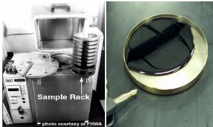
Figure 3.8 The Pressure aging vessel equipment and Sample Rack
