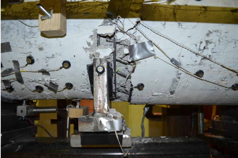
Figure 5-14: Specimen H1C1-M Shear/Local Failure at West Point of Load Application
