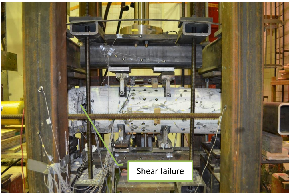
Figure 5-16: Specimen H1C2-C after Shear Failure
