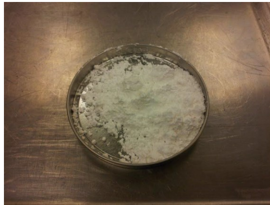
Figure 2.3. Advera Synthetic Zeolite WMA Additive for Foaming Asphalt
