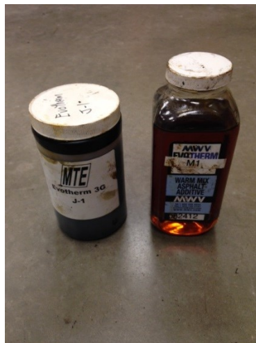
Figure 2.4. Warm Mix Additive Evotherm® J-1 and M1 Manufactured by MeadWestvaco
