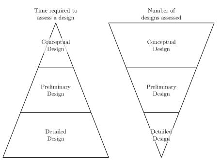
**Figure 3:** Increasing Time Requirements per Analysis Leads to Fewer Considered Designs in Progressive Stages of Aircraft Development
