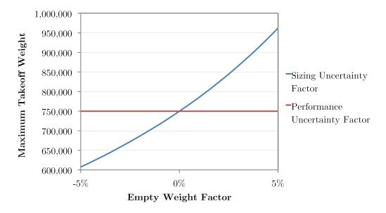
Figure 34: Change in Maximum Takeoff Weight vs. Empty Weight Factor
