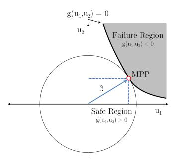
Figure 19: Most Probable Point (MPP) of Failure
