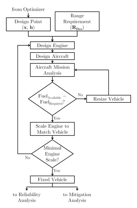
Figure 49: Vehicle Sizing Logic Flow
