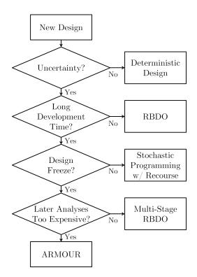
Figure 46: Establishing the Need Flowchart
