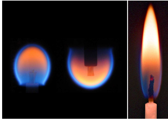
Figure J0.3. Images of a candle diffusion flame (left) in microgravity and (right) normal earth gravity [168].
