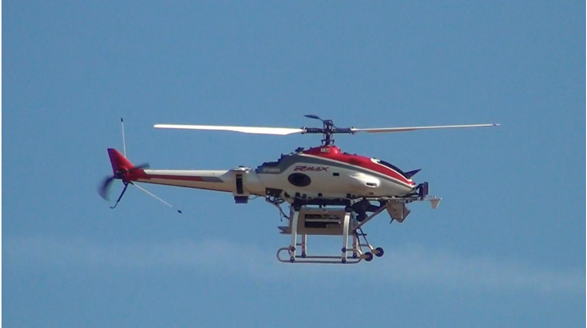
Figure 5: The GTMax helicopter weighs 80 kg and has a rotor diameter of 3 m. For vision-based navigation, a downward-facing camera is mounted on the nose of the vehicle.
