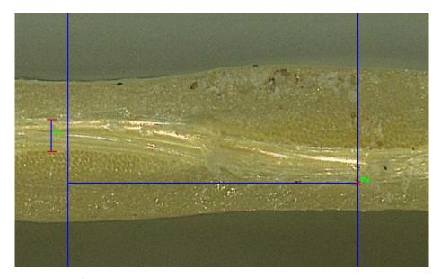
Figure C.2: Kevlar  $^{\circledR}$  49 Cross-Section Image Taken Using Keyence Digital Microscope with 150 X Magnification
