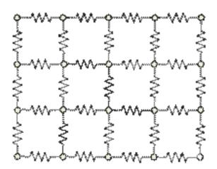
Figure 20: Example Particle-Spring Mesh [55]
