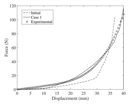
Figure 57: A Closer Match Between the Data and FEA Predictions Achieved Through the Inverse Analysis
