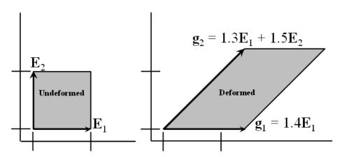
Figure 42: Determination of Deformation Gradient Graphically
