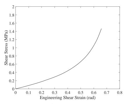
Figure B.9: 200 Denier Kevlar $^{\circledR}$  Trellis Frame Stress Vs. Strain - Ramp Up
