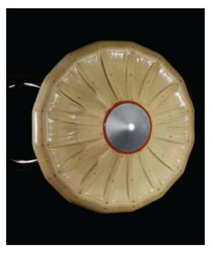
Figure 1: Inflatable Tension Cone Model (Front View) [15]
