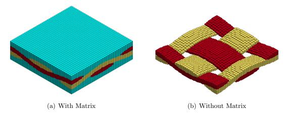
Figure 64: 8 Noded Hexahedral Elements - Voxel Mesh
