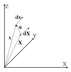
Figure 43: Element Position Vectors
