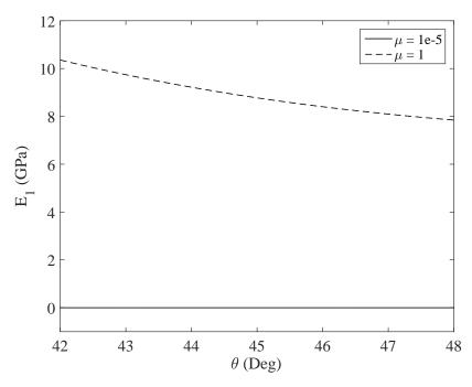
Figure 51: Comparison of Braid Angle Influence on Homogenized Longitudinal Elastic Modulus in Free and Locked States
