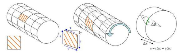
Figure 30: Inflated Cylinder - Shear Modulus Estimation [26]
