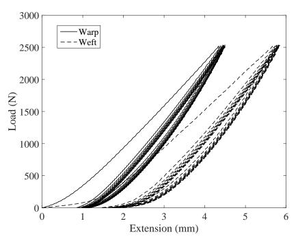
Figure 26: 200 Denier Kevlar® Warp and Weft Uniaxial Tension Test - All Ten Cycles
