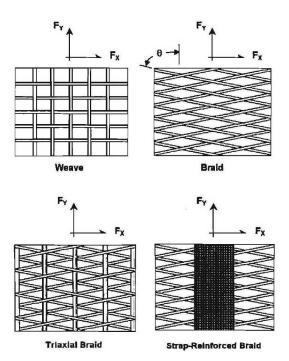
Figure 2: Example Fabric Architectures used in Air-Inflated Structures [29]
