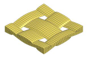
Figure 63: 8 Noded Hexahedral Elements - Volume Mesh
