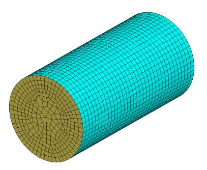
Figure 77: Inflated Cylinder Finite Element Model
