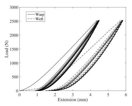
Figure B.1: 200 Denier Kevlar® Warp and Weft Uniaxial Tension Test - All Ten Cycles
