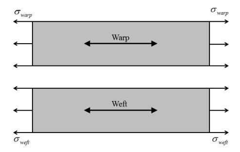
Figure 25: Textile Uniaxial Stress-Strain
