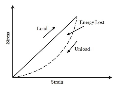
Figure 27: Idealized Uniaxial Loading Hysteresis Cycle
