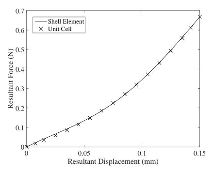
Figure 75: Comparison of Resultant Force in Pure Shear
