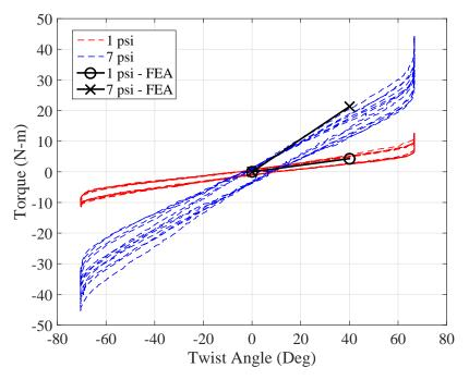
Figure 38: Applied Torque versus Twist Angle Comparison between Model and Data Cylinder of Urethane Coated Kevlar® at Three Inflation Pressures
