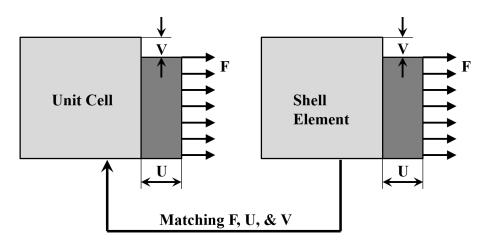
Figure 73: Equivalent Membrane Element in Uniaxial Tension
