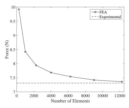
Figure 33: Applied Load (N) Vs Number of Elements
