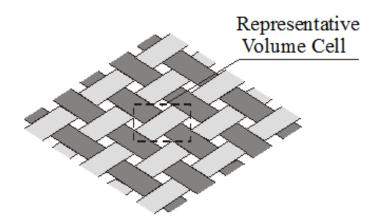
Figure 39: Flexible Woven Interlacing Pattern [64]
