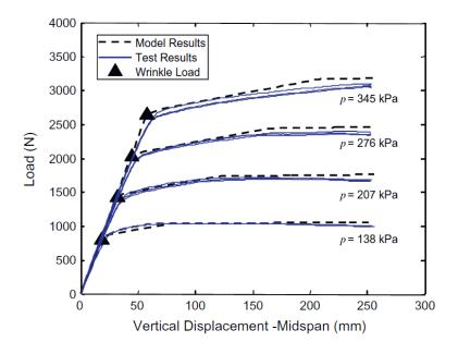
Figure 9: Air Beam Four-Point Bend Test Results [35]
