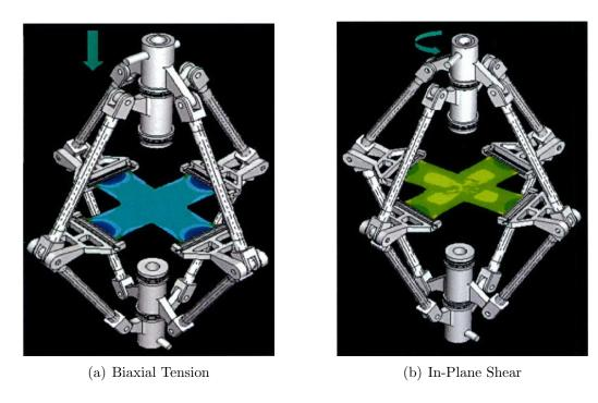
Figure 15: Combined Biaxial Tension and In-Plane Shear Test Methods [44]
