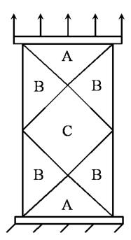
Figure 28: Bias Extension Deformation Zones
