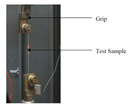
Figure 3: Yarn Tensile Testing using Instron®
