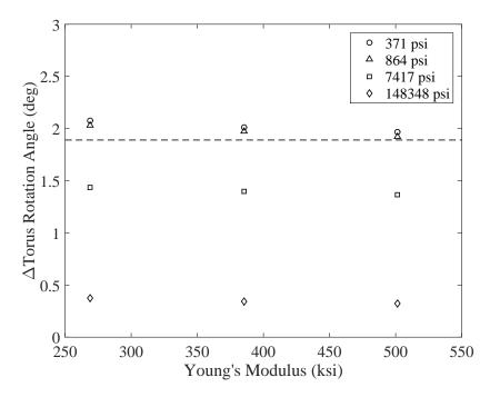
Figure 79: Comparison Between Change in Tension Cone Torus Angle for Various Shear and Elastic Moduli. Dashed Line Corresponds to Experimentally Observed Torus Rotation of 1.89°
