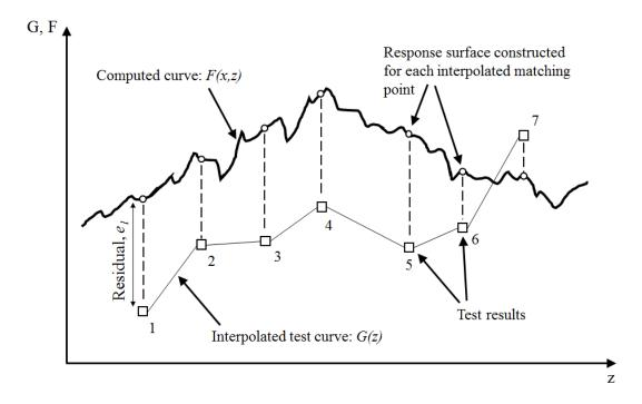
Figure 24: Components of Mean Square Error Formulation
