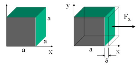
Figure 65: Cube of Material Under Uniaxial Tension
