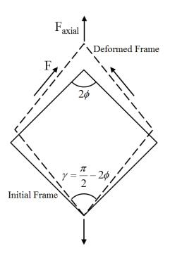
Figure 29: Trellis Frame - Shear Modulus Estimation
