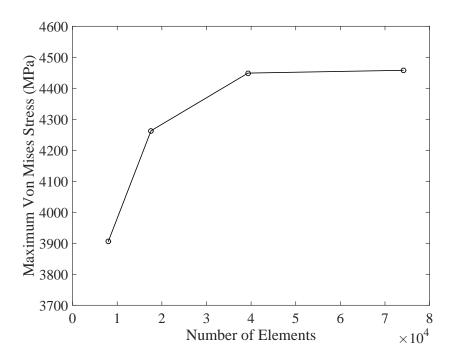
Figure 68: Von Mises Stress Vs. Number of Elements
