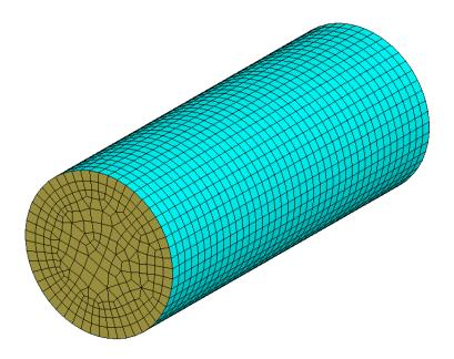
Figure 37: Inflated Cylinder Finite Element Model
