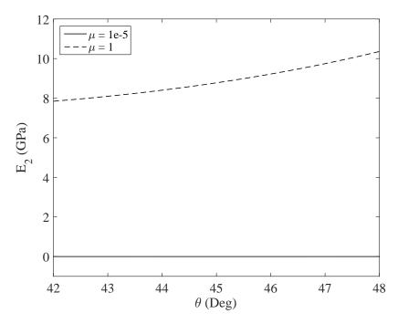
Figure 52: Comparison of Braid Angle Influence on Homogenized Transverse Elastic Modulus in Free and Locked States
