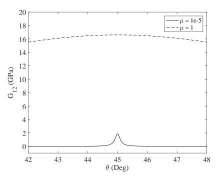
Figure 54: Comparison of Braid Angle Influence on Homogenized In Plane Shear Modulus in Free and Locked States
