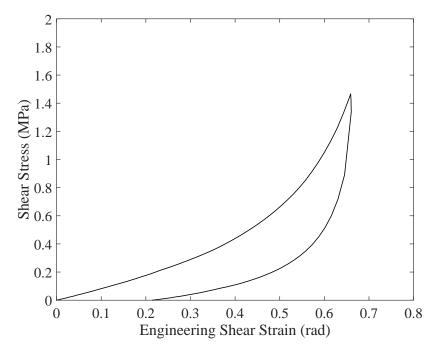
Figure B.8: 200 Denier Kevlar® Trellis Frame Stress Vs. Strain
