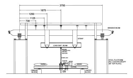
Figure 8: Air Beam Four-Point Bend Test Diagram [35]
