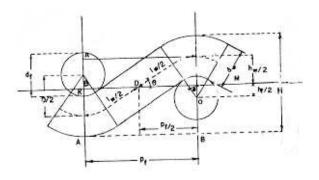
Figure 4: Fabric Geometric Model [33]
