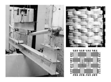
Figure 18: 4-Point Beam Bending and Fabric Sections
