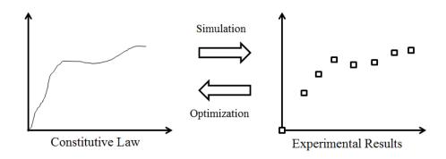
Figure 22: Material Identification Process
