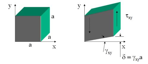
Figure 66: Cube of Material Under Shear Stress
