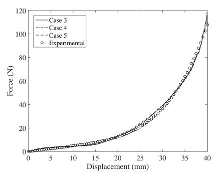
Figure 58: Close Agreement Between the Data and FEA Predictions Achieved Through the Inverse Analysis with Subset of Parameters
