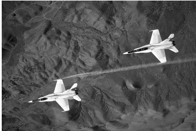
Figure 13: F/A-18 Autonomous Formation Flight Project - NASA Dryden Research Center
