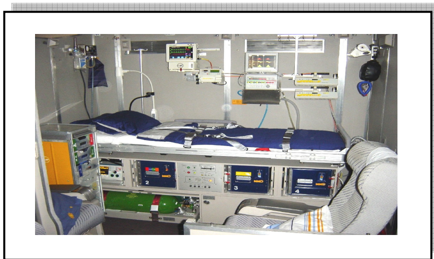
Picture 2.11: Example of a customised and fully equipped patient transport compartment
