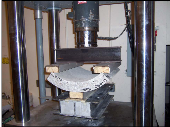
Figure 3.3 Three-point bending process used to generate cracks on the interior surface of the pipe quadrant specimens
