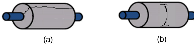
Figure 4.14 Illustration of observed orientations of induced cracking. (a) longitudinal and (b) circumferential, both across cylinder half, as a result of uniform and localized corrosion morphology along embedded rebar, respectively.
