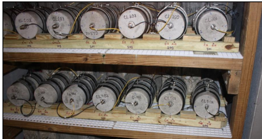
Figure 3.12 Test specimens under impressed current in a controlled RH chamber
