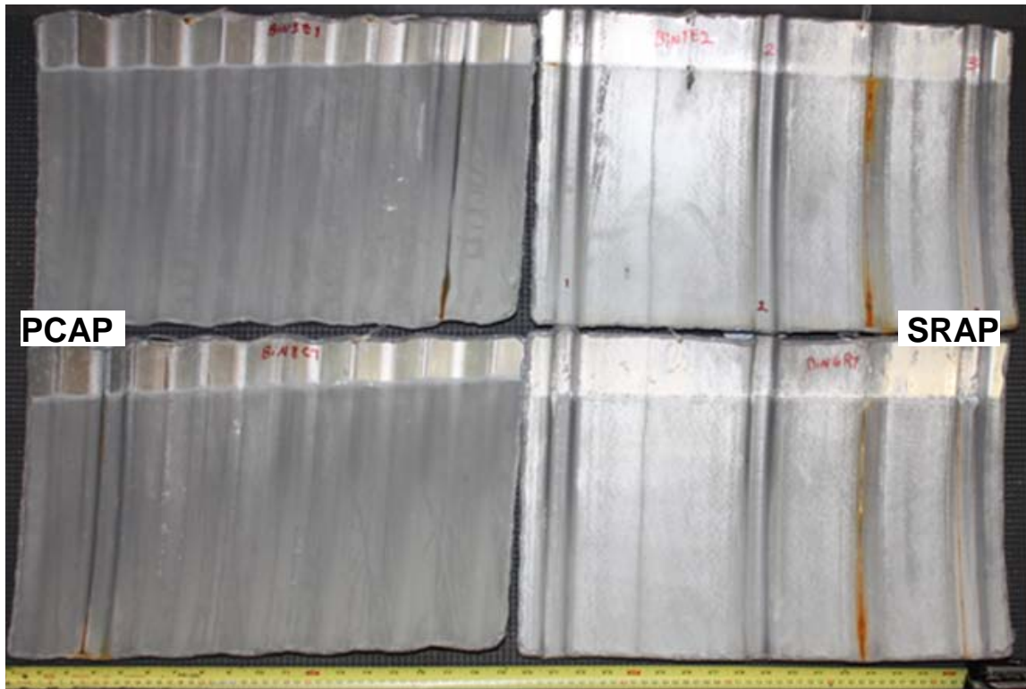
Figure 31: PCAP and SRAP specimens in solution S (Top) and S + (Bottom) after ~700 days of exposure (specimens internal ID code: Bin 1 E2 (Top-right), Bin 6 R7 (Bottom-right), Bin 3 E1 (Top-left) and Bin 8 C7 (Bottom-left)).
