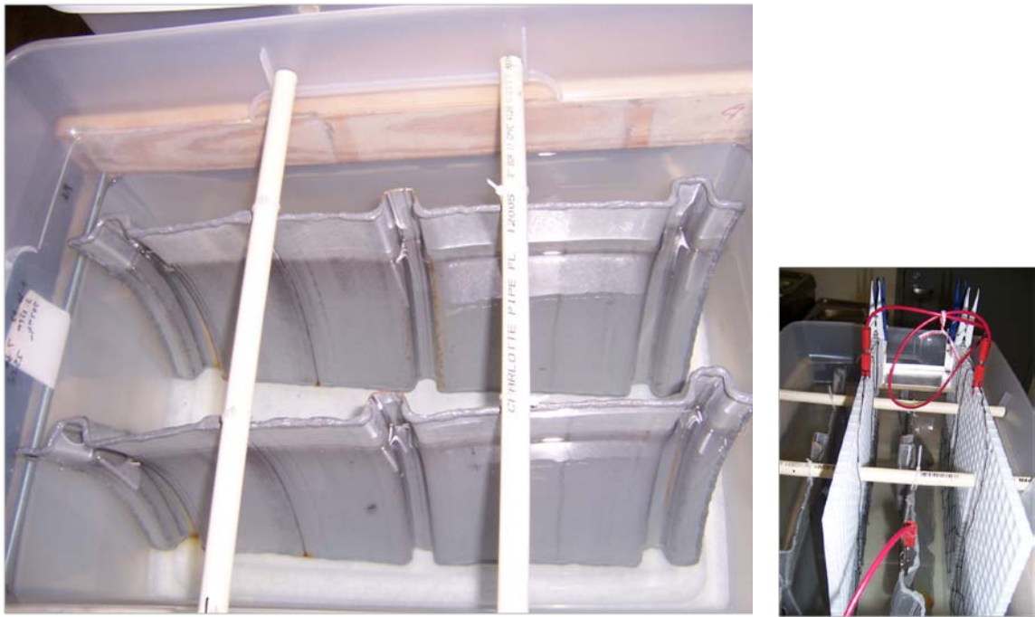
Figure 30: Large SRAP specimens in a large bin (Left). Up to 5 cm of the top of the specimens were not immersed. Counter electrode inserted during EIS tests (Right).
