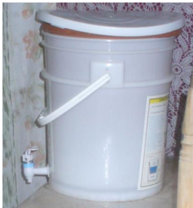
Figure S-1 Photo of a distorted lid that does not adequately cover the filter.
