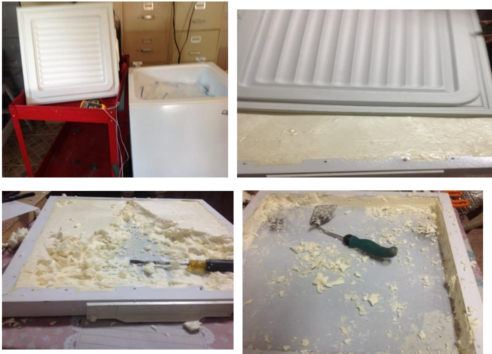
Figure 3.6 After the traditional testing was conducted, the cover was removed and the external plastic sheet was removed. The internal metal sheet was pried from between the plastic sheet and the polyurethane manually.
