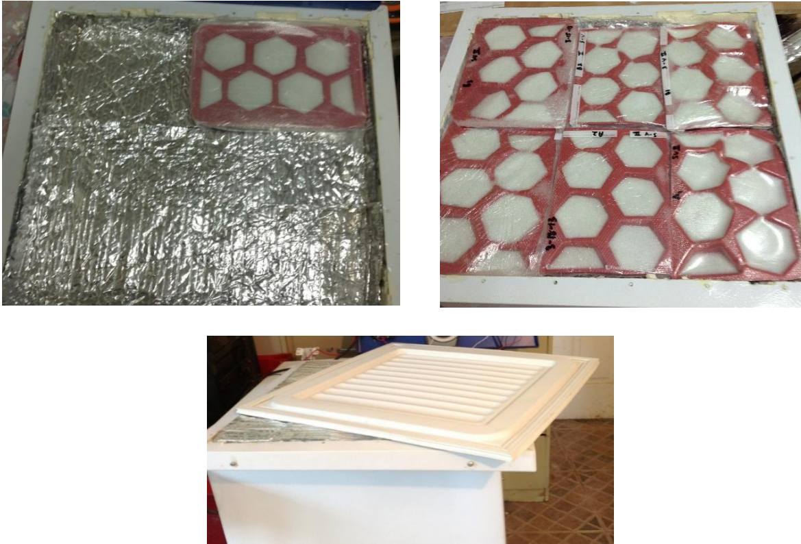
Figure 3.7 The polyurethane insulation from Unit A was manually stripped and the metal sheeting was pried apart from the external plastic sheath. The reflective heat shield was inserted, followed by the thermoformed pastic insulation cartridges contained packets of evacuated silica. The insulation cartridges was split into six parts due to limitations of manufacturing, and then joined using epoxy resin.
