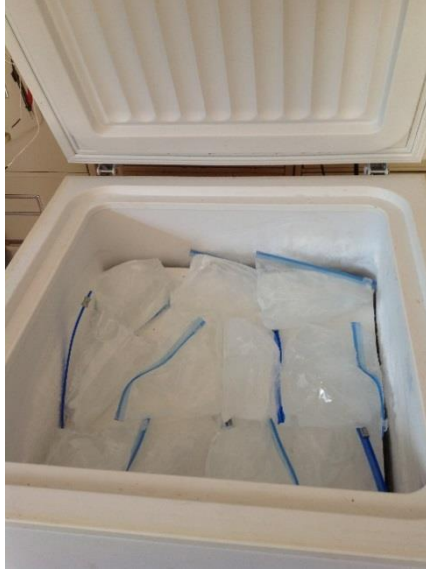
Figure 3.9 Testing of Unit A. Testing protocol (ASHRAE 72-2005) states that test units must be filled with saline packets to simulate real world conditions.
