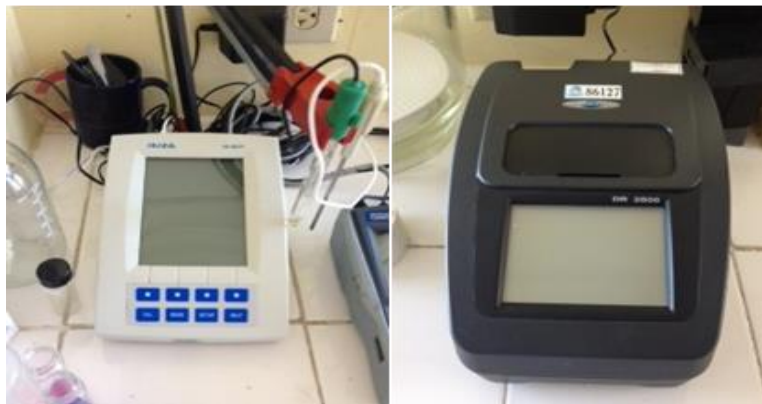
Figure D.7: (a) HANNA HI 4211 Bench Meter (Ann Arbor, MI) (b) HACH Spectrophotometer DR 2800
