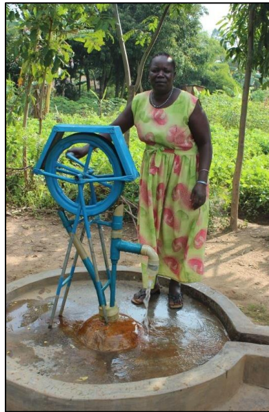
Figure 6: Self-supply borehole, Rope Pump, and owner in Gulu, Uganda (Photo: Author)
