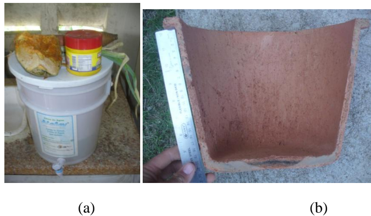
Figure 1. The Potters for Peace (PFP) Ceramic Pot Filter. (a) A PFP filter in its bucket at a household in the field. (b) A cross-sectional view of the PFP filter.
