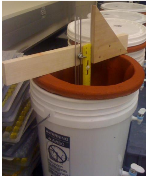
Figure 5. The T Device. The horizontal wood piece fixes the height of the ruler in the filter. The drop in water height after one hour corresponds to the amount of water filtered.
