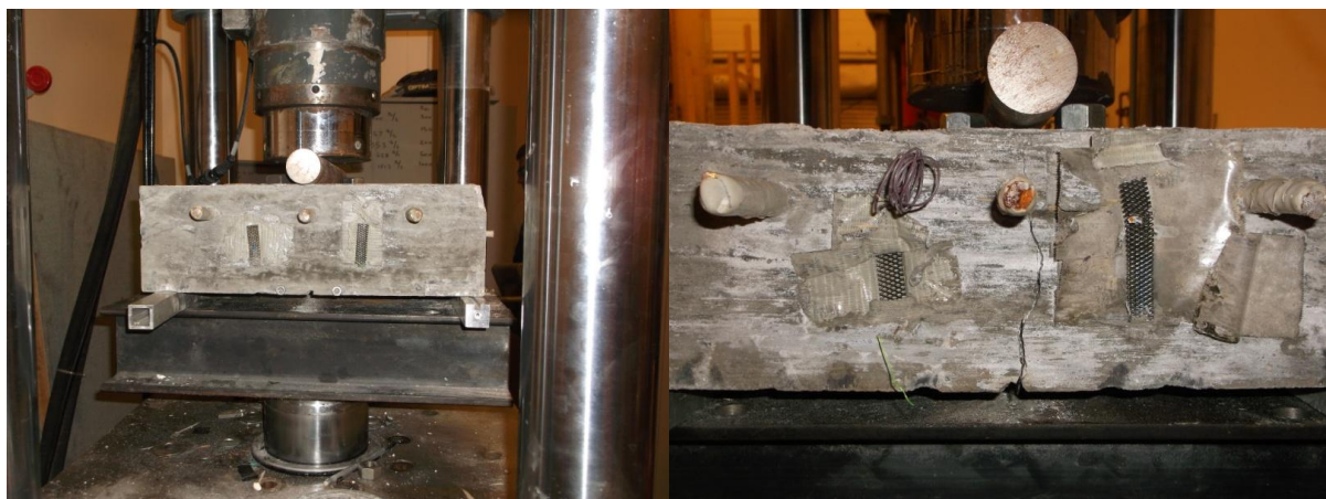
Figure 8 Three Point Bending Test Configuration
