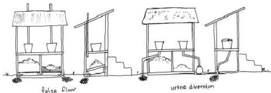
Figure 4: Two-vault composting latrine. Source: Figure from Mihelcic et al. (2009) with permission provided by Linda A. Phillips.
