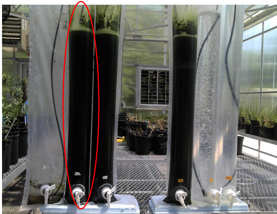
Figure 14-Tubular photobioreactors located in greenhouse (Halfhide, 2011)
