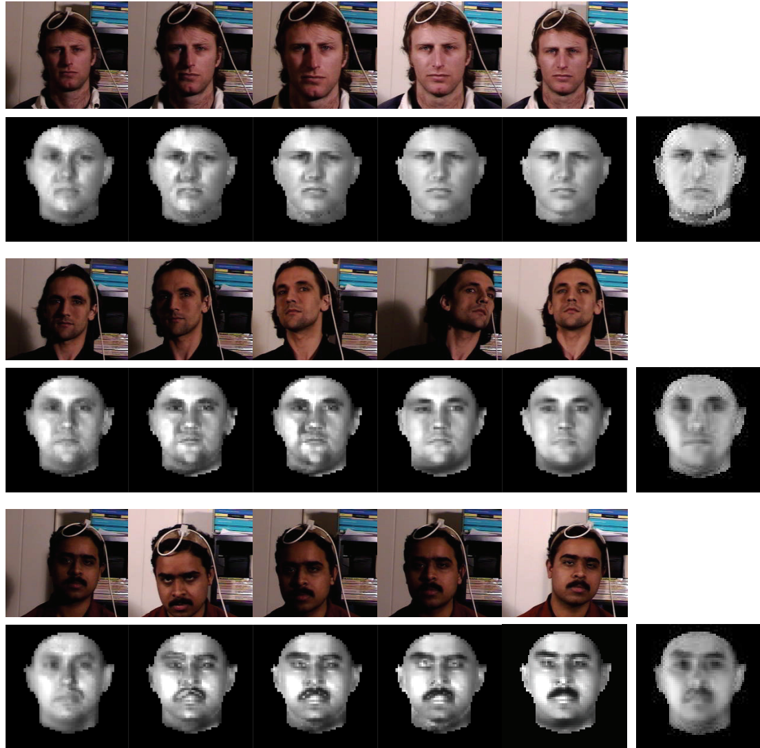
Figure 2.9: Albedo maps estimated for three sequences in the BU dataset. The rows show some of the frames in each sequence followed by the estimated albedo using the proposed algorithm up to that frame. The last column shows the averaging of the estimated albedos obtained using [1] at each frame.
