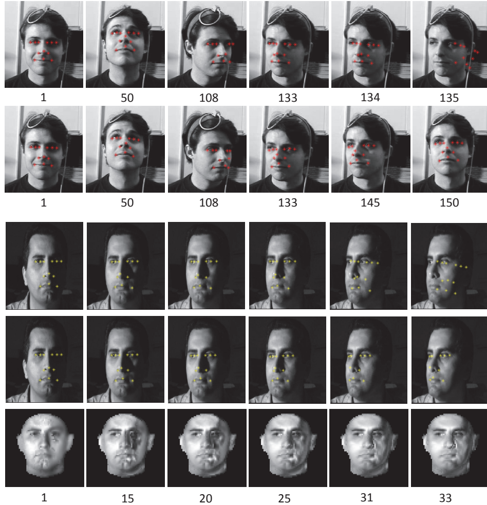
Figure 2.13: Comparing the pose tracking results with and without albedo updating step. For each sequence, the first row shows the tracking results of the particle filter without the albedo updating step and the second row has the results of the proposed algorithm. For the second sequence, we also show the estimated albedo map using the proposed algorithm at each frame. The frame numbers are shown below images.
