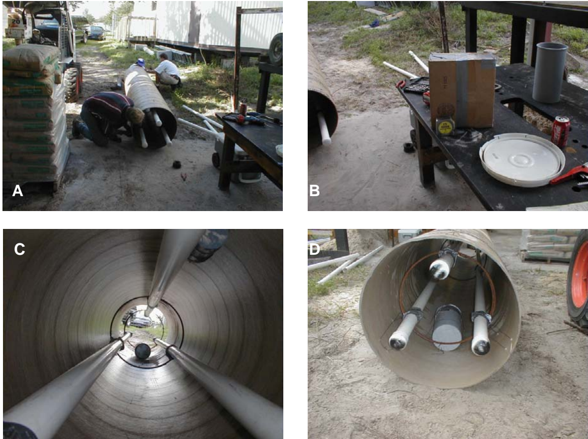
Figure 4.11 - Placing anomalies for field trial #1, A - inserting and securing access tubes and ties, B - example of anomaly sand box, C - inside of Sonotube showing anomalies, access tubes and ties, D - end or bottom view of replica shaft showing access tubes and anomaly
