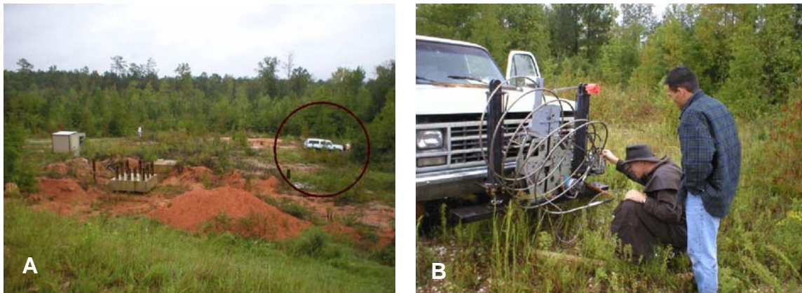
Figure 5.2 - Alabama site soil testing, A - CPT soundings in test area, B - subsurface exploration using the USF mini-CPT rig
