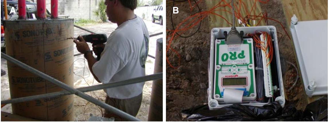
Figure 4.31 - Installing thermocouples for field trial #2, A - insertion of 2-wire thermocouples, B - data logger for thermocouples
