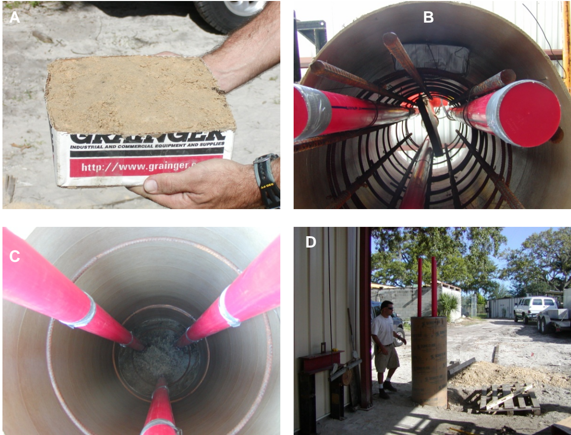
Figure 4.30 - Field trial #2 test set-up, A - sand box anomaly, B - anomaly and cage inside of Sonotube, C - erected control shaft top view, D - erected control shaft elevation view
