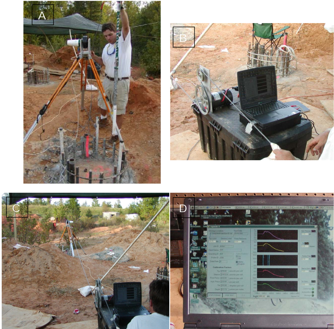
Figure 5.22 - TIP testing at Auburn test site, A - tripod, depth wheel, tripod and down hole sensor, B - driver motor and pulleys, signal conditioning and portable computer, C - overall test setup, D - screen shot showing real time thermal sensors
