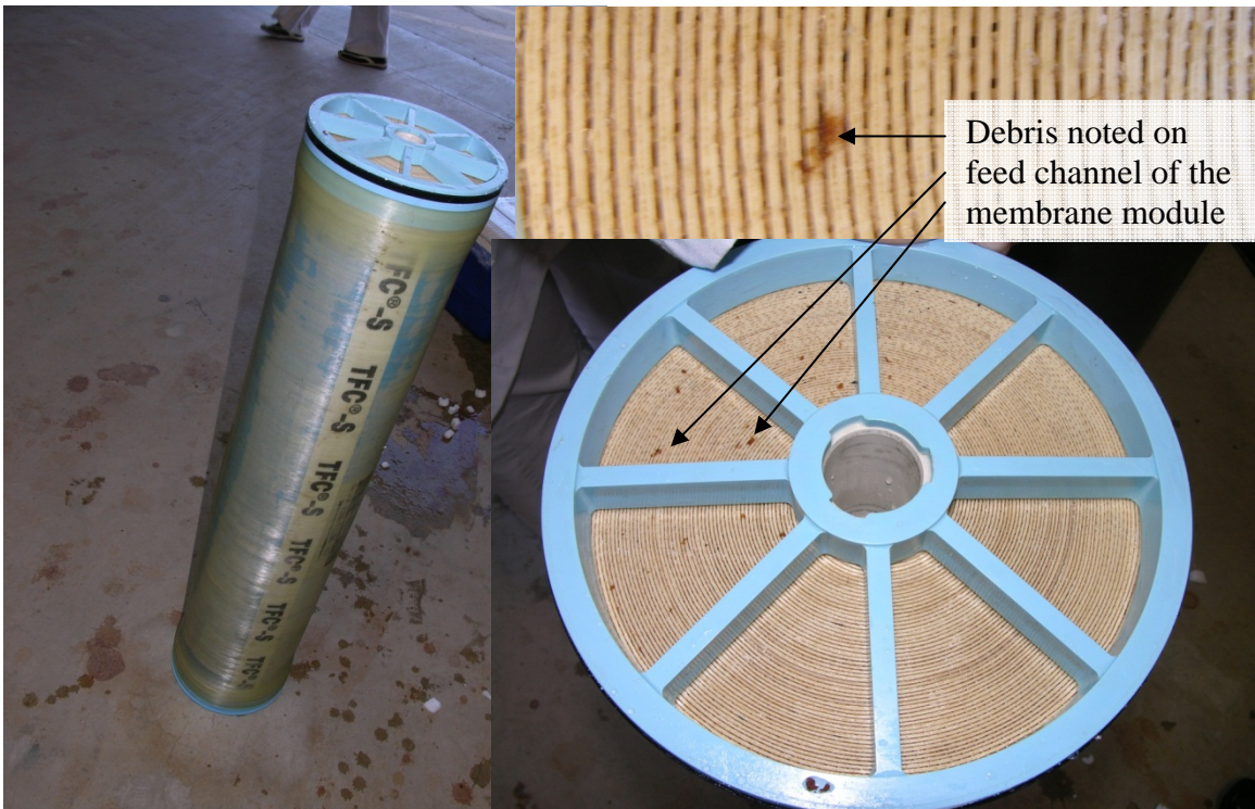
Figure 5-1 Membrane element autopsied in Orange County showing the feed channel with debris deposited
