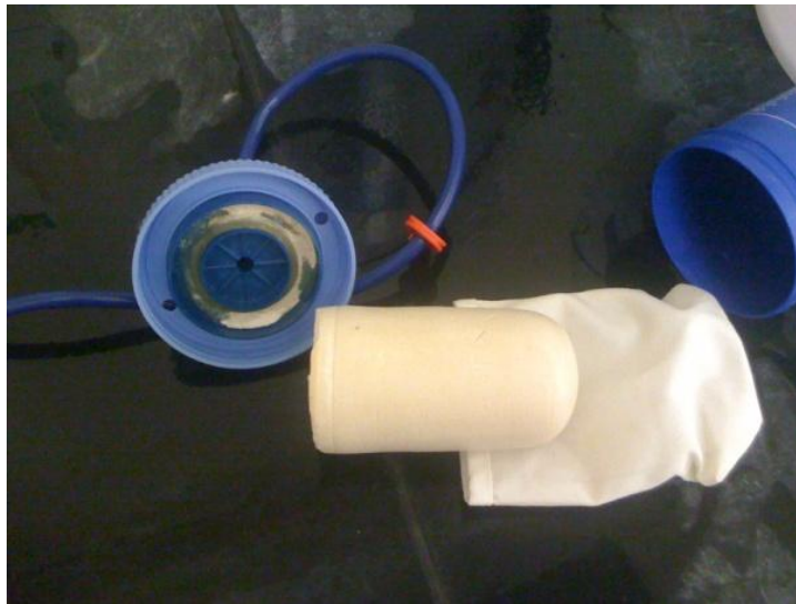
Figure 12. Filter 7 after the glue failed. At this point Filter 7 was taken out of the experiment.
