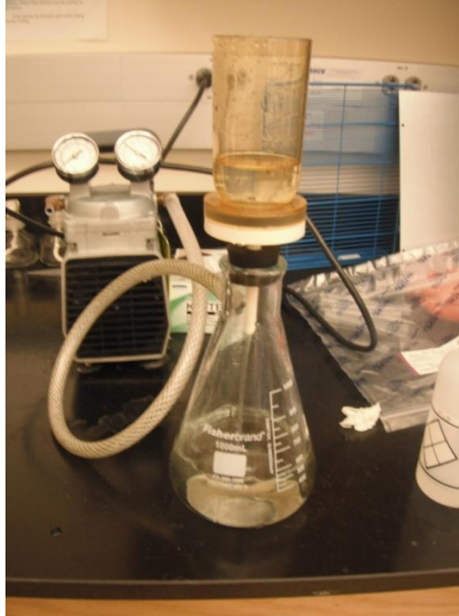
Figure 9. Total suspended solids (TSS) set-up pictured here. The vacuum pump pulls water from the top through the dried glass microfiber filter. The glass filter is weighed before and after the sample is run. By using the difference in weight and the volume of the water processed, the total suspended solids can be determined.
