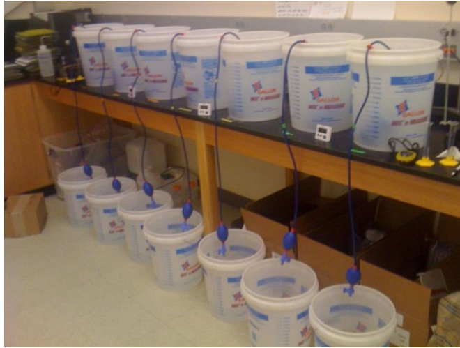
Figure 5. Initial set-up with all seven filters sitting in 20 L buckets and dispensing into 20 L buckets below. On the far left is the control filter with increasing turbidities from left to right.
