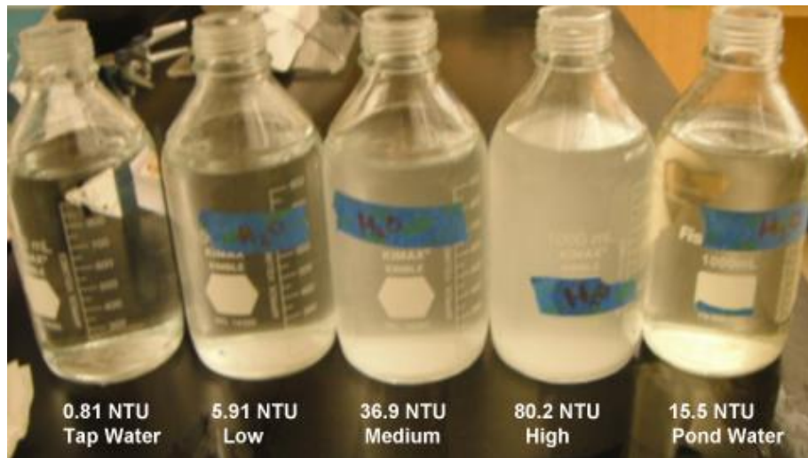
Figure 13. Influent samples after settling for 30 minutes. From left to right, the first is tap water (average 0.81 NTU), then low turbidity water (average 5.91 NTU), medium turbidity water (average 36.9 NTU), high turbidity water (average 80.2 NTU), and pond water (average 15.5 NTU).
