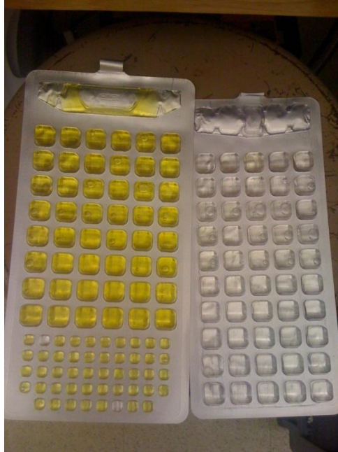
Figure 8. IDEXX Colilert® results. On the left is a Quanti-Tray® /2000 showing a positive result for total coliforms of influent pond water from Filter 4. There are 48 positive large wells (out of 48 total large wells) and 46 positive smaller wells (out of 48 total smaller wells) which result in a most probable number of 913.9 CFU. On the right there is a sample of effluent water of Filter 4 in a Quanti-Tray®. This sample has zero positive wells which correlates to a most probable number of <1 total coliform forming units.
