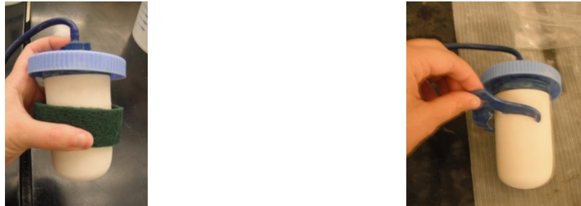
Figure 11. Scrubbing ceramic candle using the green scrubbing pad. On the right, shows measuring the ceramic candle to ensure that it is still going to effectively remove pathogens.
