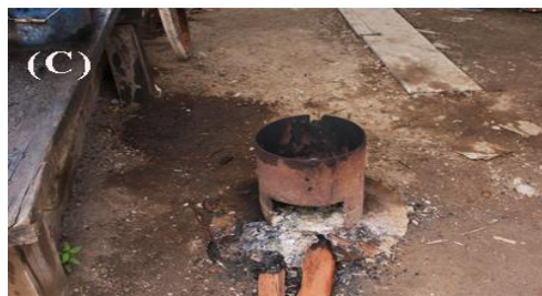
Figure 7.10. Mercury Use at a Mine in Mahdia, Guyana with Posters Done by the GENCAPD Project in Conjunction with the Guyana EPA. (A) Mercury is Stored in a Safe Place, (B) A Retort with the Amalgam Heated Over a Fire in a Closed Container and the Vapors Collected Under Water, (C) Retort is Burned in a Fireplace in the Mining Camp.
