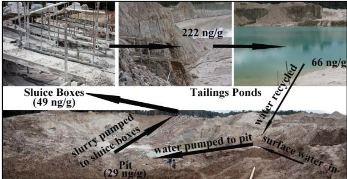
Figure 4.8. Diagram of Mine 2 in Mahdia, Showing Main Mining Processes and Areas Sampled Including: 1) The Pit Where High Pressure Water is Used to Make A Slurry With the Ore; 2) Sluice Boxes Fitted With Mats That Trap Gold Bearing Ore As Slurry Passes Over; and 3) Tailings Ponds Where Sediment is Allowed to Settle, Sometimes With the Help of Flocculants.
