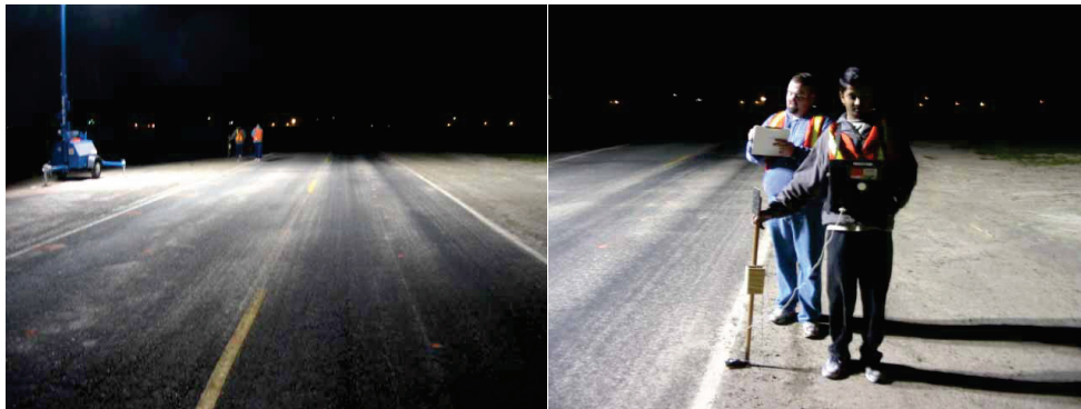
Figure 2 Example of Traditional Roadway Lighting Illuminance Measurements
