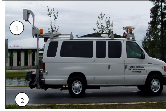
FIGURE 20(a) FDOT Multi Purpose Survey Vehicle (MPSV) Used for Pavement Imaging
