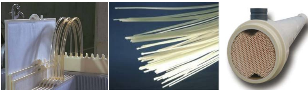
Figure 2.9 Flat Sheet, Hollow Fiber and Multi-Tubular Membranes [44-46]
