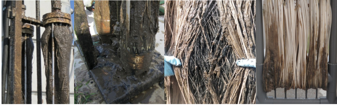
Figure 2.13 Examples of MBR Membrane Fouling
