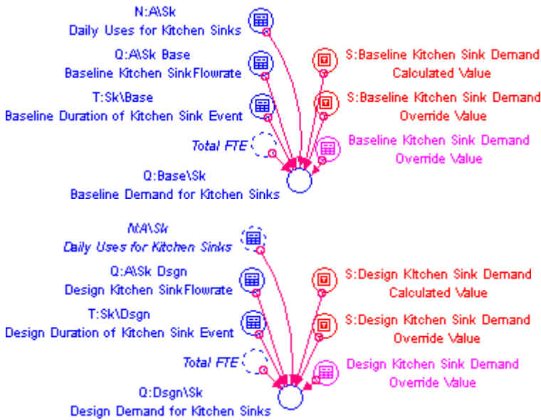
FIGURE A5: Baseline (top) and design (bottom) components for kitchen sinks in the IBWM model.
