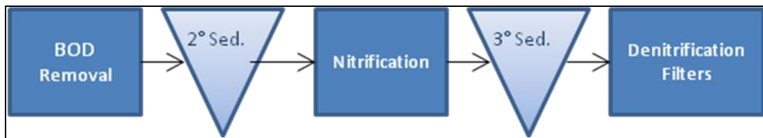
Figure 4. Schematic of the section of the treatment process at the HFCAWTP modeled in this study. Sedimentation basins were not considered individually, but removal rates due to settling were considered.
