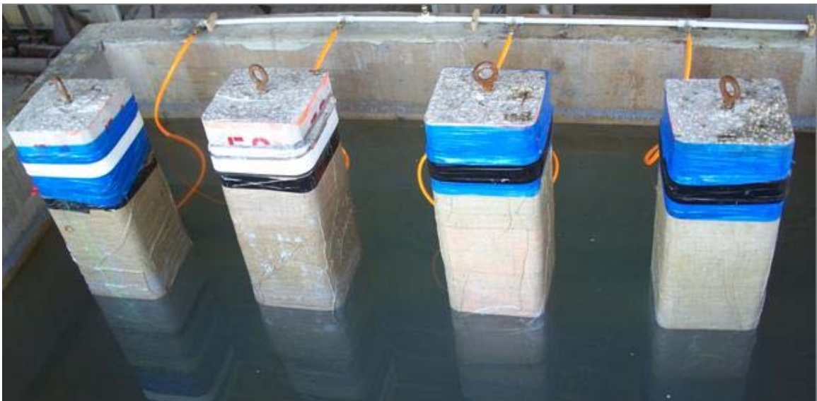
Figure 3.3 Vacuum bagged repaired piles.
