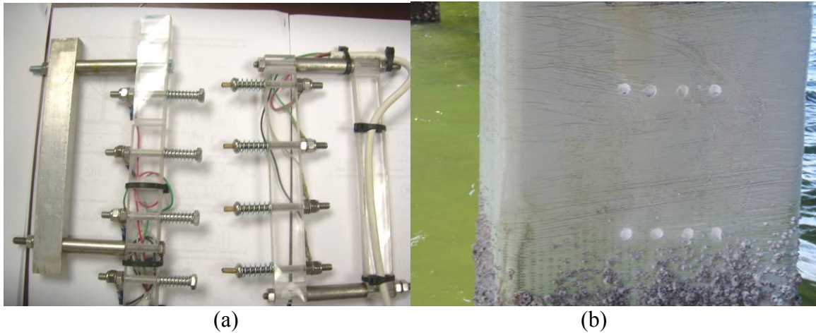
Figure 2.15 (a) Resistivity probe; (b) Holes in FRP for concrete resistivity testing.
