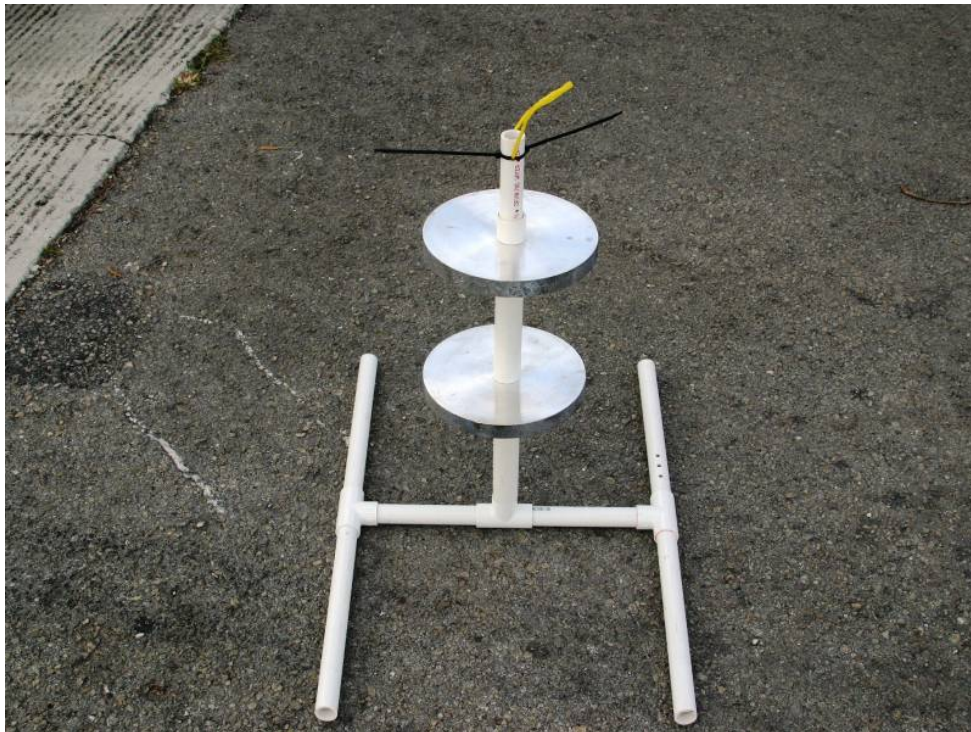
Figure 5.12 Magnesium specimens mounted on stand prior to submersion.
