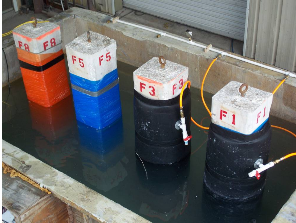
Figure 3.1 Control and pressure bagged piles.
