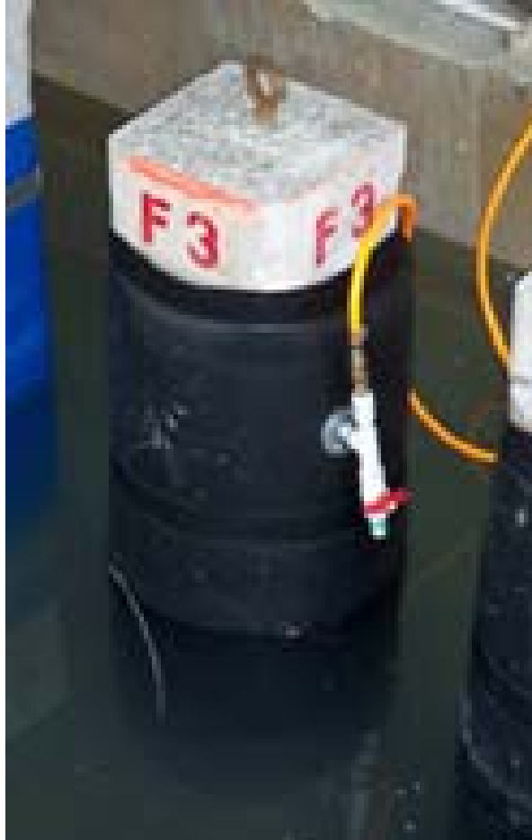
Figure 2.5 Pressure bagged pile.
